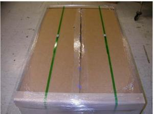
3.4 Place two pallet labels (33G6283) one on the front and one on the left sides of the pallet load.
