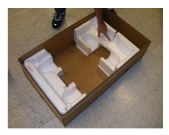
2.8 Place load spreader (32R0212) inside the bottom void in the rear of the unit. Assemble and place load spreader (32R0211) inside the entire void in the rear of the unit. Care should be taken to insure that Corrugated load spreader (32R0211) fully engages the side covers of the unit. Tape the Corrugated load spreader to the side covers of the unit with (4) four 152mm pieces of Strapping Tape (01R3747).
