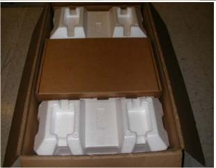
2.22 Close the top of the carton and seal with printed tape. (74F5699 - Automatic taper, 74F5698 - for hand held dispensers)
