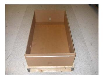
2.4 Locate and brake apart all three sections of bottom cushion set (01R4022). The front section of the cushion
