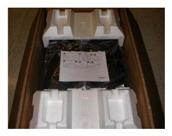
2.21 Assemble Tower Shipgroup carton #2 (01R4040). Place keyboard and mouse inside carton. Place carton in center cavity between the top cushions. (Scan shipgroup cart #2 Barcode if prompted by DFC)
