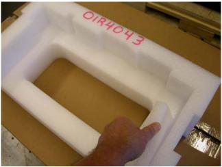
2.20 Place top cushions on unit. Make sure the top front cushion (01R4043) is on the front of the unit and the top rear cushion (01R4044) is on the rear of the unit.
