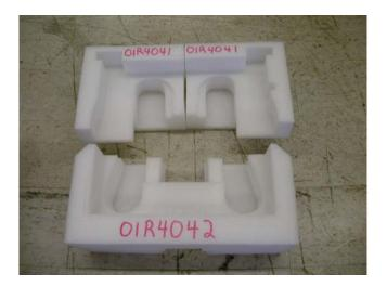
2.5 Remove tear-outs sections from both sides of bottom front cushion (01R4041) and bottom rear cushion (01R4042).
