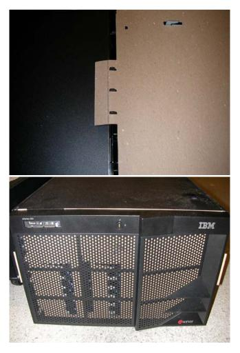
2.10 Place PolyBag (37L0557) over top of unit. Once bag is on, tuck one end of the bag under the unit between the front and rear wheels and pull through to the opposite front and rear wheels, eliminating any slack in the bag. Place IBM logo tape on end of bag that was pulled through under the unit and seal shut.
