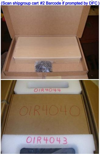
2.23 Close the top of the carton and seal with printed tape. (74F5699 - Automatic taper, 74F5698 - for hand held dispensers)
