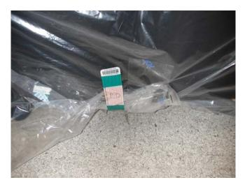
2.12 Place unit in bottom cushions. Make sure system in positioned all the way down and not sitting on the cushion ledge.
