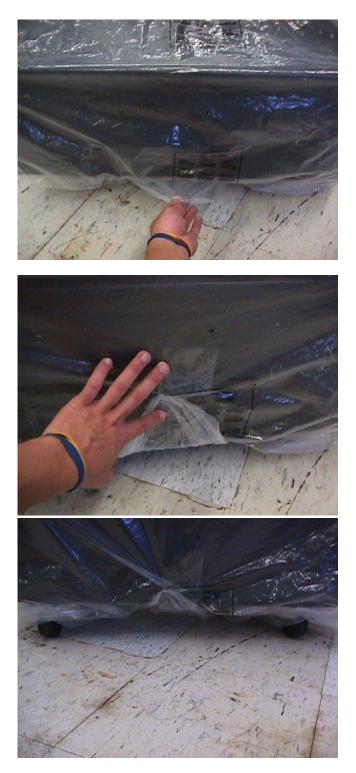
2.11 Place tamper label (06P6550) on bag vertically (as shown) next to previously placed IBM logo tape to seal edge of fold over bag.
