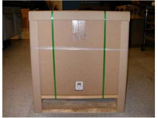
3.3 Stretch wrap the unit to the pallet utilizing Best of Breed" methods. The Stretch wrapping Machine MUST wrap a minimum of three times around the base and four times around the top of the load with 100% coverage of the product using the roping technique. If roping capabilities are not available you Must use palletization Methods 2 or 3 as outlined in documents 92F6168 "Best of Breed" Pallet Unitization or QMX document P-04146.
