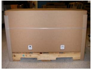
3.2 Place one 24 inch corner board on each of the two short top edges of the package and two way band the unit to the half-pallet.
