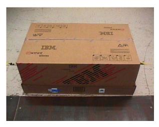
2.24 Take the two (2) printed carton labels (33G9780) off the printer. Position labels on front and left sides of the carton using label locating marks.
