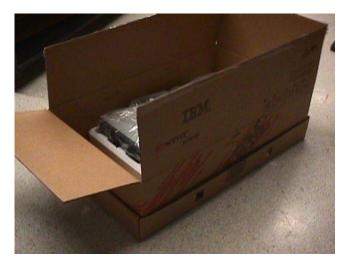
2.11 Place corrugated clip (6X) (37L0511) into square holes in bottom tray and snap shut. Insure that clips go through carton and tray securing carton and tray together.
