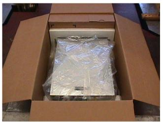
2.16 Break apart top cushion set (25P1116) and place on top front and rear edge of system.
