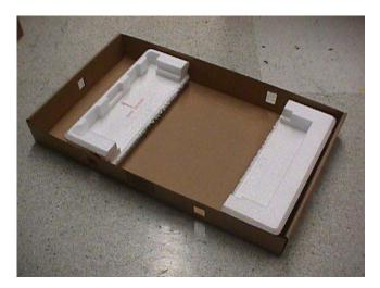
2.6 Leave about 5 inches of space for the shipgroup between the edge of the bottom tray and edge of front bottom cushion. The arrow (colored in red for clarity)on the front bottom cushion must always point toward the shipgroup.
