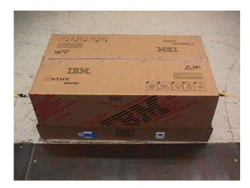
2.21 Take the two (2) printed carton labels (33G9780) off the printer. Position them on front and left sides of the carton. Use label locating marks.
