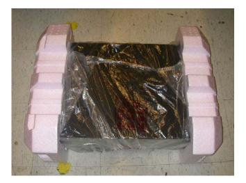
2.7 Place system into carton with left side up (latch up), sliding the system all the way back until the rear cushion is in contact with the rear wall of the carton.
