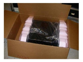
2.8 Insert corrugated insert (32R0093) in front of the system. Bend flaps of insert back at 45 degree angle around the front cushion (shown in red).
