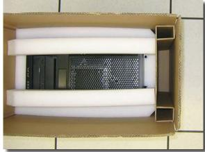
2.11 - Insert keyboard box into the compartment of filler. Skip this step if there's no keyboard bundled.
