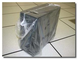
2.4 - Fold bag over, and seal bag closed with 06P6550 padlock label. (illustrated below).
