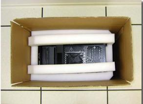
2.10 - Fold cardboard filler 40K9255 and insert it into the space at the bottom of chassis. Note the hand hold is on top.
