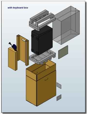
2.1 - Assemble carton 40K9253 and tape the bottom flaps shut as shown.
