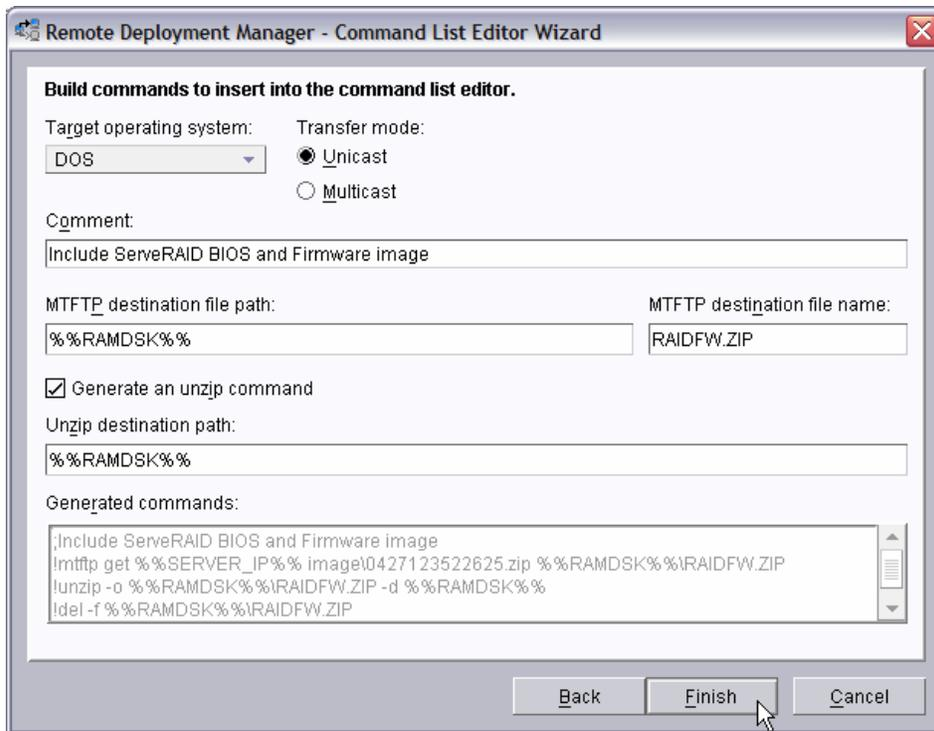
18. Enter the appropriate data to generate the correct commands to download and unzip the custom image you created in section 3.2 above.
