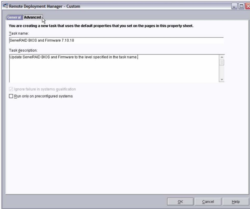
14. Enter the task information on the General page (e.g., name the task *ServeRAID BIOS and Firmware 7.10.18*). Notice that we include the version number in the task name. That’s because the task is tied to a particular BIOS/firmware version. If, later, a new BIOS/firmware version becomes available, you will probably create a new task to deploy the newer version.
