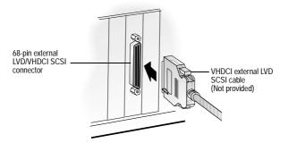
**2** Connect the other end of the cable to a SCSI connector on the back of an external device. If you are installing only one external device, terminate the device and skip to Step 4.
