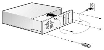
**3** Locate an unused 64-bit PCI/PCI-X expansion slot and remove the expansion slot cover. If the computer does not have a 64-bit slot, you can install the card in a 32-bit PCI slot. The Adaptec SCSI Card 29320LP supports both 5V and 3.3V 64-bit slots. (The expansion slot must be compliant with PCI Rev. 2.2 or PCI-X Rev. 1.0 and must support Bus Mastering.) Save the slot cover screw for use in Step 4.
