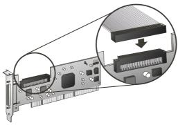
**3** Plug the internal Ultra320/160 and Ultra2 SCSI devices to the other cable connectors, starting with the connector at the terminated end of the cable.
