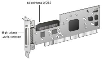
Although the Adaptec SCSI Card 29320LP is a 64-bit PCI/PCI-X card, it also works in a 32-bit PCI slot. When installed in a 32-bit PCI slot, the card automatically runs in the slower 32-bit mode.
