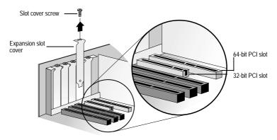
Computers may have vertical or horizontal expansion slots. Refer to your computer manual to locate the PCI/PCI-X slots. If your computer is a tower model, lay it on its side to allow for easier installation of the Adaptec SCSI Card 29320LP.
