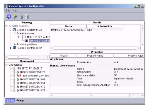
Figure 37. Displaying information about one remote I/O enclosure
