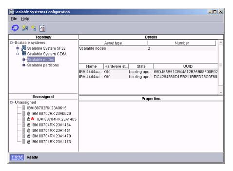
Figure 30. Displaying information about all scalable nodes in one scalable system
