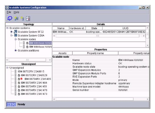
Figure 32. Displaying information about one scalable node
