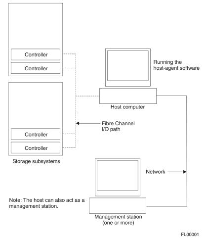
Figure 1. Host-agent (in-band) managed storage subsystems
