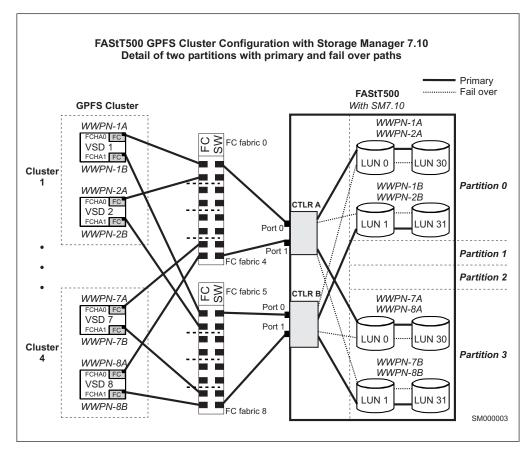
Figure 16 illustrates a FAStT500 configured with two partitions and two GPFS clusters.
