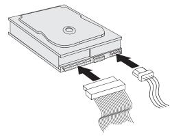
Attach an available connector on the SCSI cable to the connector on the hard disk drive, as shown. If you are connecting your new drive to a SCSI adapter that has 68-pin D-shell connectors, the connector is narrower at the top and will fit only one way.
