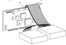
Remove any terminators or terminating jumpers on devices in the middle of the chain.
