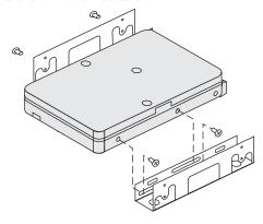
These brackets are available in the IBM 3.5-inch to 5.25-inch conversion kit, IBM part number 70G8165. Refer to the documentation that comes with the conversion kit for instructions on using the expansion brackets.
