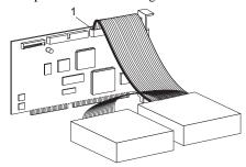
Remove any terminators or terminating jumpers on devices in the middle of the chain.
