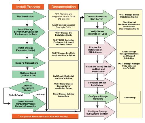
Figure 1. Installation process flow by current publications
