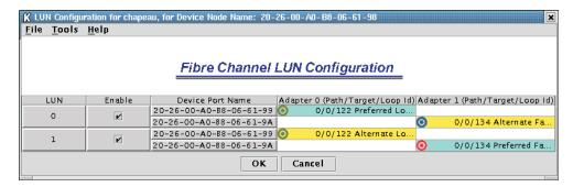
Figure 80. Preferred and alternate paths between adapters
