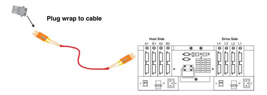
Figure 60. Install wrap plug
