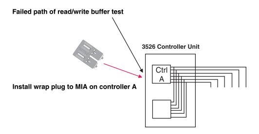
Figure 105. Install wrap plug to MIA
