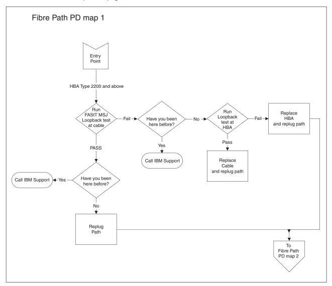
For information about how to run loopback tests, see Chapter 4, "Introduction to FAStT MSJ," on page 55.
