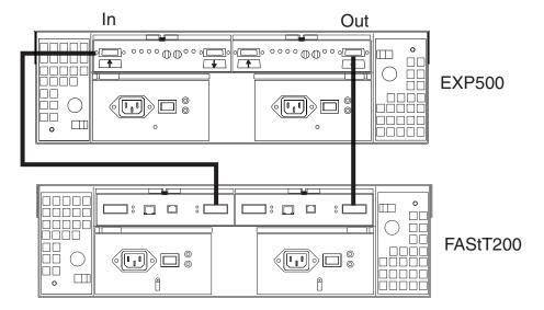
Figure 70. EXP500 and FAStT200 configuration
