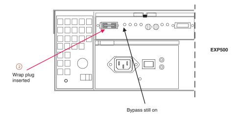
Figure 86. Insert wrap plug
