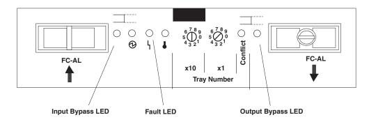
Figure 95. FAStT EXP500 ESM indicator lights
