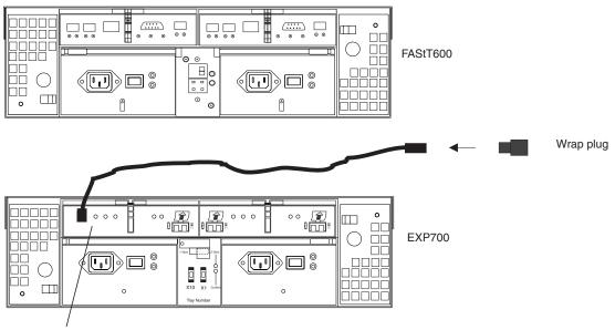
Record status of bypass light after wrap plug is inserted.
