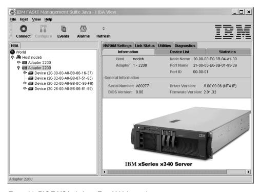
Figure 61. FAStT MSJ window - Two 2200 host adapters
