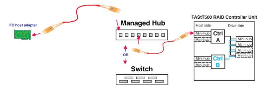
Figure 101. Typical connection path
