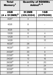
This table does not represent all possible memory configurations. RDIMMs must be added in sets of four to support interleaving technology.
