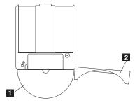
To return the disc to the cartridge, align the label side of the disc **1** with the DVD-RAM cartridge label side. Insert the disc and close the cartridge lid **2**. A clicking sound will occur when the lid closed.
