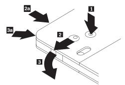
Using the tip of a ball point pen, push and break the lock pin tab **1**. To remove the disc, use a ball point pen to push down on the cartridge lid lock **2** and pull the cartridge lid out **3**. When the cartridge lid is open, the disc can be removed.
