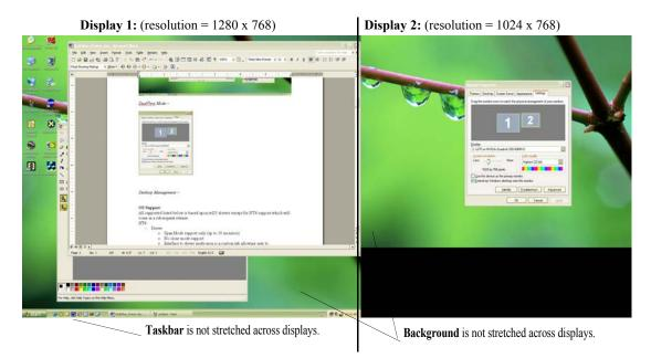
Figure 3.4 Multiple Display Devices in nView Dualview Mode
