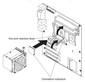
1. Make sure that the microprocessor socket lever and cover are in the fully open position.
