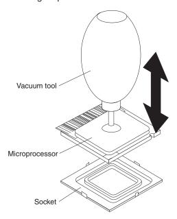
a. Squeeze and hold the bladder of the tool; then, place the suction cup on the microprocessor and release the bladder.
