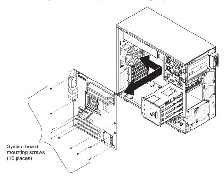
1. Insert the system board into the chassis and slide it toward the rear of the server until it fully engages the tabs in the chassis.
