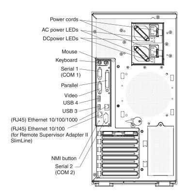
The following illustration shows the input/output (I/O) connectors on the rear of the non-hot-swap power supply models.
