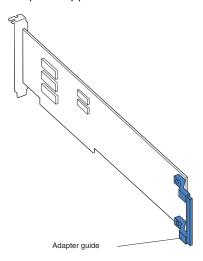
8. Carefully grasp the adapter by the top edge or upper corners, and align it with the expansion slot guides; then, press the adapter *firmly* into the expansion slot. Move the adapter directly from the static-protective package to the expansion slot.
