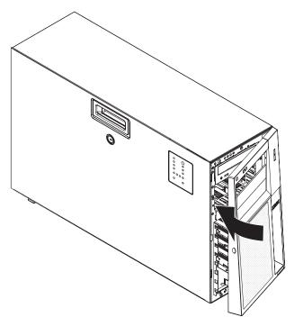
2. Rotate the bezel toward the server until it snaps in place.
