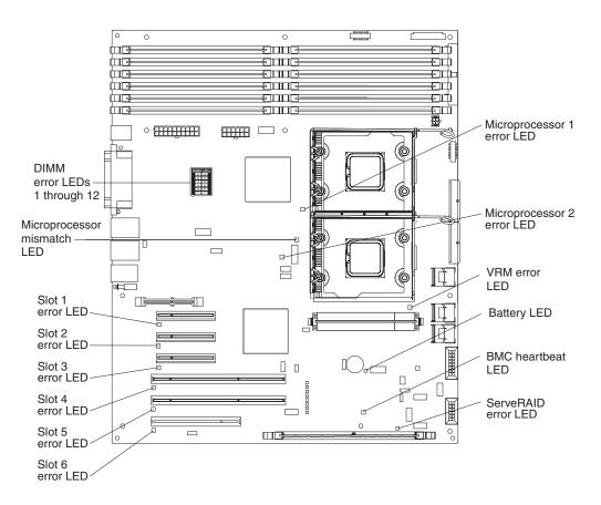
Use the system-board LEDs to diagnose system errors. An error LED is lit to indicate a problem with a specific component. After a problem is corrected, the LED will not be lit the next time that the server is restarted; if the problem remains, the LED will be lit again. For additional information, see the *Problem Determination and Service Guide* on the IBM *System x3400 Documentation* CD.
