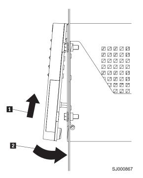
Figure 10. Replacing the controller unit bezel (machine types 3552 and 1742)
