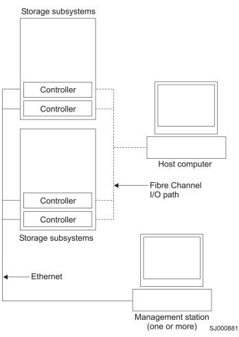
Figure 3. Direct (out-of-band) managed storage subsystems
