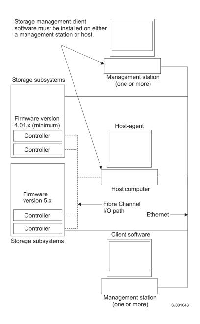
Figure 6. Coexisting storage subsystems
