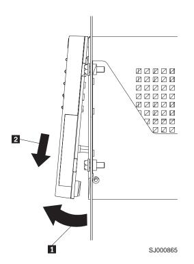
Figure 9. Removing the controller unit bezel (machine types 3552 and 1742)
