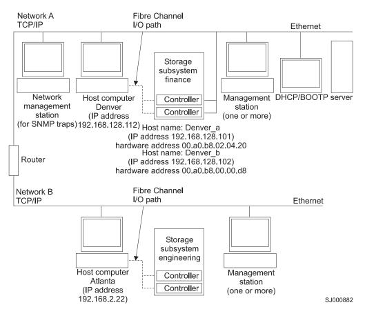
Figure 7. Sample network using direct-managed and host-agent-managed storage subsystems
