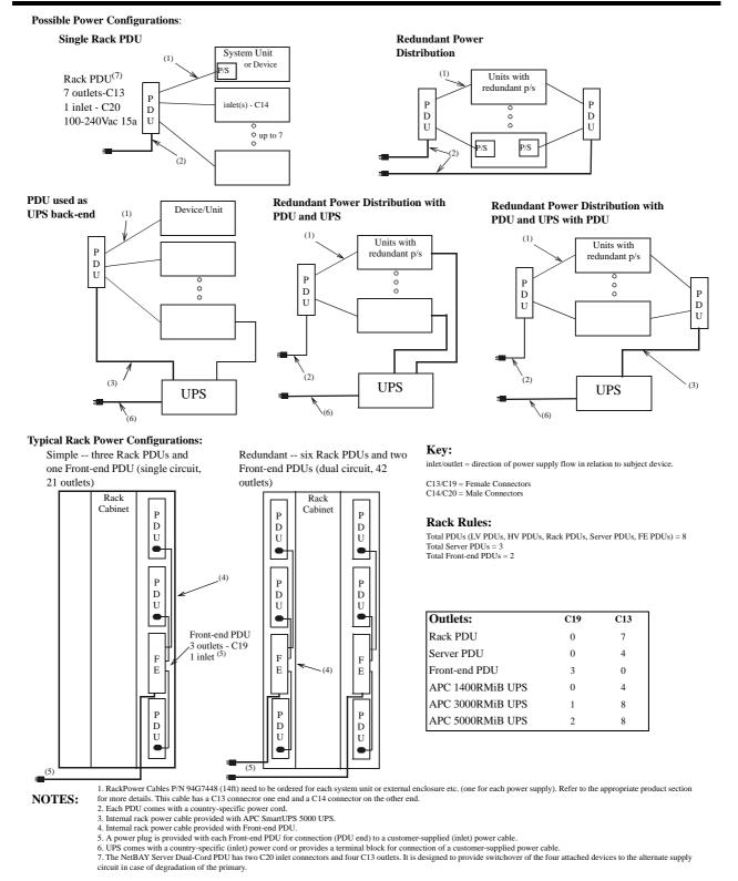
Note: the Customer is required to provide a dedicated power supply circuit for each line cord protected with an appropriate circuit breaker
