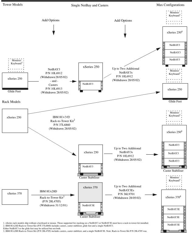
JBM 80/X28D Rack-to-1ower Kit (P/N 28L4/05) includes casters, caster stabilizer, and a single NetBAY 3E. Note: Rack-to-1ower Kit P/N 28L4/05 was withdrawn from marketing on 31/12/01.
