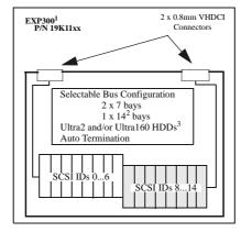
1. Housed in a 19in rack mountable drawer and ships standard with redundant 500 W hot-swap power supplies, two power cords and a single 2M Ultra2 SCSI cable capable of supporting Ultra160 Speeds.
