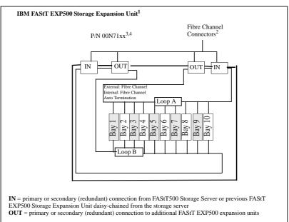
1. Housed in a 19" Rack mountable drawer and ships standard with redundant power supplies and two standard country power cables requiring separate power sources. Requires IBM industry standard 19" rack, EIA-310D, with a minimum depth of 24" (711.2 mm) or NetBAY3/3E.
