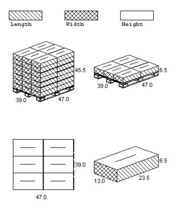
2.1.2 - Secure load to pallet utilizing "Best of Breed" palletization methods. See 92F6168
