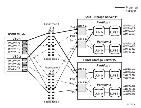
Figure 18. RVSD cluster configuration with two FAStT storage servers — two partitions per FAStT
