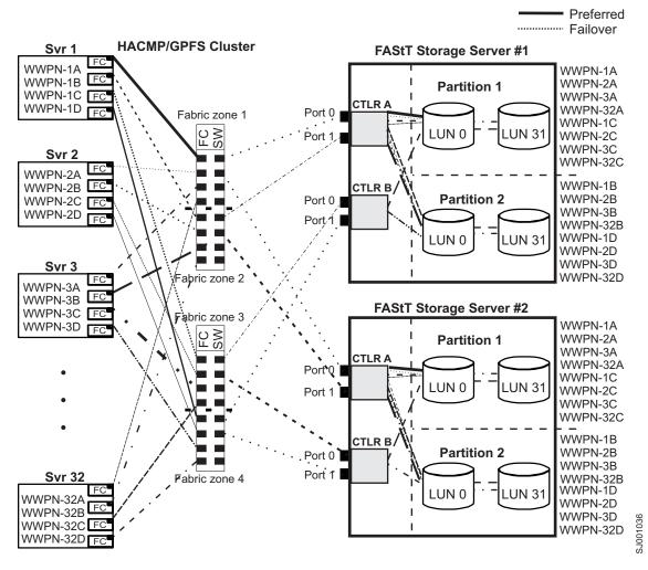
Figure 20. HACMP/GPFS cluster configuration with two FAStT storage servers — two partitions per FAStT
