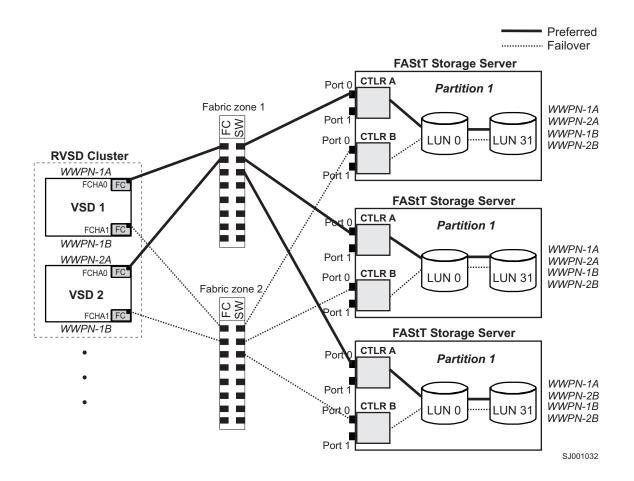
Figure 16. Cluster configuration with three FAStT storage servers — one partition per FAStT
