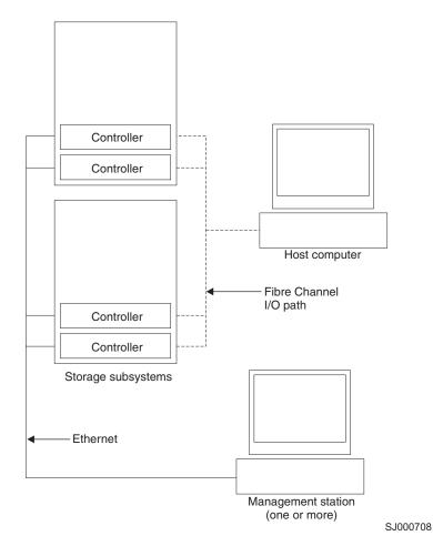
Figure 3. Direct (out-of-band) managed storage subsystems
