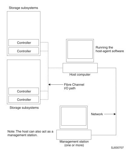
Figure 2. Host-agent (in-band) managed storage subsystems
