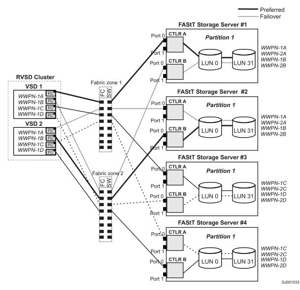
Figure 17. Cluster configuration with four FAStT storage servers — one partition per FAStT
