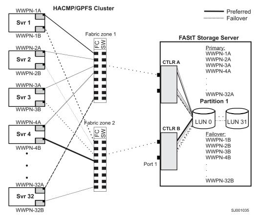
Figure 19. HACMP/GPFS cluster configuration with one FAStT storage server - one partition
