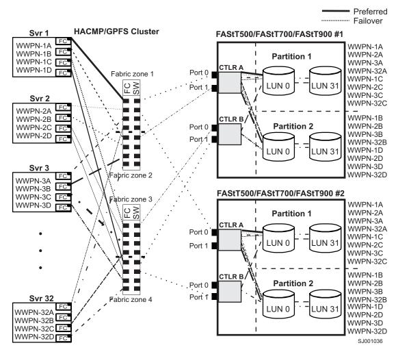
Figure 19. HACMP/GPFS cluster configuration with multiple FAStT500/700/900, shown with two partitions per FAStT
