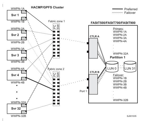
Figure 18. HACMP/GPFS cluster configuration with single FAStT500/700/900, shown with one partition per FAStT
