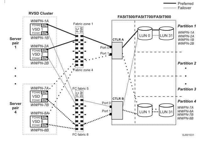
Figure 14. RVSD cluster configuration with single FAStT500/700/900 - Storage Manager 8.3, shown with two partitions (four maximum) per FAStT
