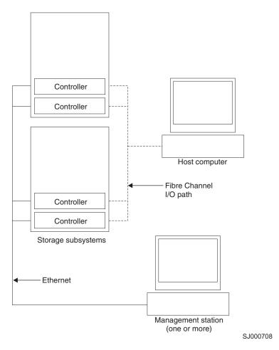
Figure 3. Direct (out-of-band) managed storage subsystems
