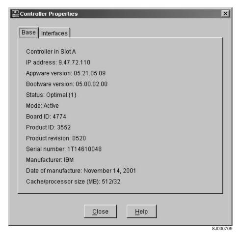
Figure 4. Controller Properties window
