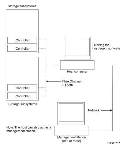
Figure 2. Host-agent (in-band) managed storage subsystems
