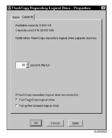
Figure 44. Repository drive warning threshold
