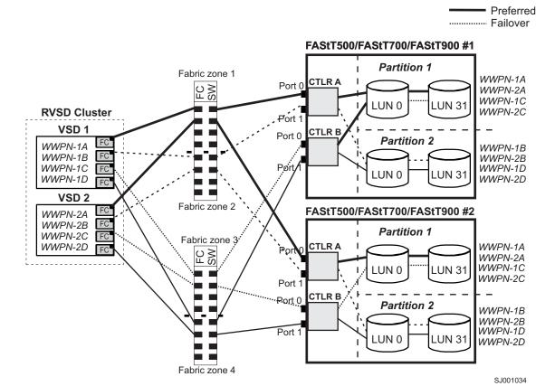
Figure 17. RVSD cluster configuration with multiple FAStT500/700/900 - Storage Manager 8.3, shown with two partitions per FAStT
