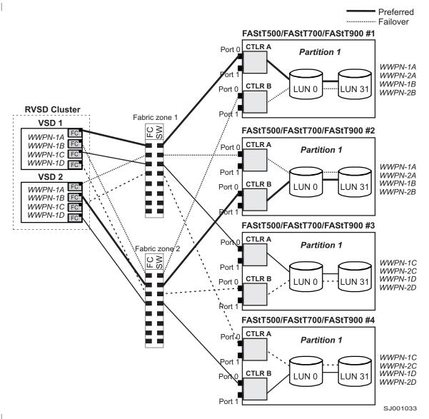
Figure 16. Typical RVSD cluster configuration with multiple FAStT500/700/900 - Storage Manager 8.3, shown with one partition per FAStT
