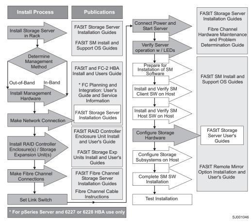
Figure 1. Installation process flow by current publications
