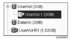
Figure 47. Icon showing the disabled FlashCopy logical drive
