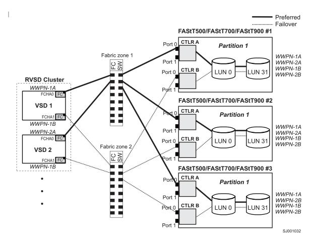
Figure 15. RVSD cluster configuration with multiple FAStT500/700/900 - Storage Manager 8.3, shown with one partition per FAStT
