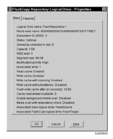
Figure 20. FlashCopy repository logical drive properties
