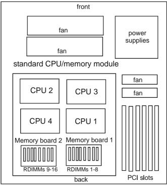
Optional SMP Expansion Module P/N 32P8340. Installs directly above standard CPU/memory board. Requires a minimum of four RDIMMs (not included).
