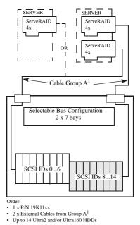
1. One 2 M Ultra2 cable is included with each EXP300. If a longer cable is desired, select one from cable group A.
