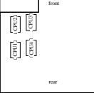
1. Three additional processors may be installed, providing a maximum of four. All processors must be identical in type, speed, and cache size. See diagram for order of installation. 2. Requires removal of the standard processor. A maximum of four processors may be installed (see xSeries 255 system board diagram
