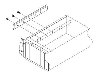
**4.** Attach the adjustable rear-rack rails to the front-rack rails. (The four  $10-32 \times 1/2$ -inch screws and nuts are provided in the miscellaneous hardware bag.)
