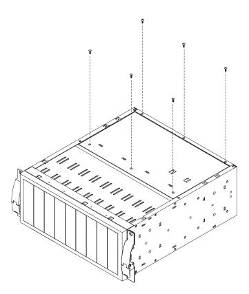
**3.** Install the slide rails on the enclosure. (The six  $10-32 \times 3/8$ -inch screws are provided in the miscellaneous hardware bag.)
