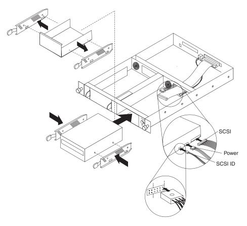
8. Install the cover on the enclosure; then, tighten the thumbscrew to secure the cover.
