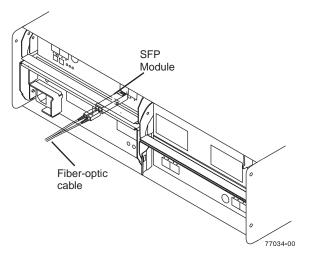
Figure 6. SFP module and fiber optic cable
