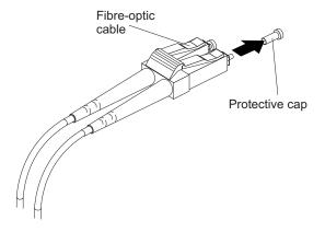
Figure 28. Removing fiber-optic cable protective caps
