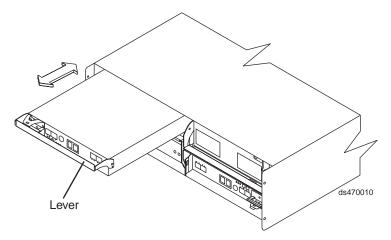
Figure 14. Removing and replacing a controller
