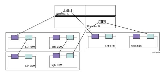
Figure 42. One DS4200 Express and three storage expansion enclosure — Recommended cabling
