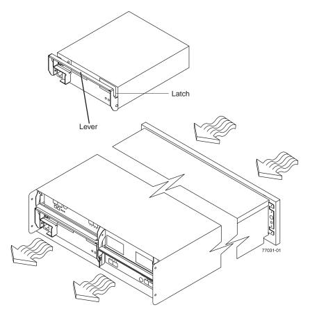
Figure 4. Power supply and fan unit and airflow
