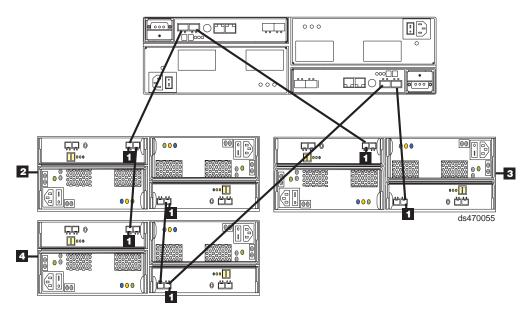
Figure 48. One DS4200 Express and three EXP420 storage expansion enclosures behind a pair of DS4200 Express drive ports
