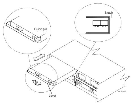
Figure 19. Removing and replacing a controller
