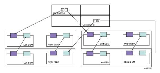
Figure 43. One DS4200 Express and four storage expansion enclosure — Recommended cabling
