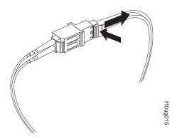
Figure 36. Removing the LC-LC fibre-channel cable from an LC-SC fibre-channel cable adapter
