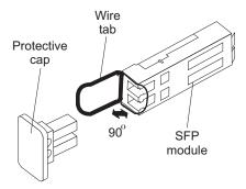
Figure 26. Unlocking the SFP module latch - wire variety
