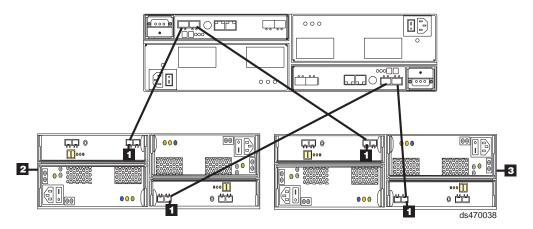
Figure 47. One DS4200 Express and two EXP420 storage expansion enclosures behind a pair of DS4200 Express drive ports
