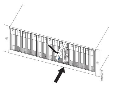
Figure 16. Removing a EV-DDM CRU
