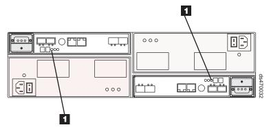
Figure 67. Cache Active LEDs
