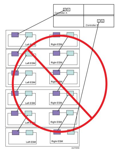
Figure 45. One DS4200 Express and up to six storage expansion enclosure — Not recommended
