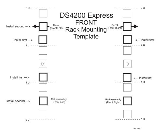
Figure 11. Front rack mounting template
