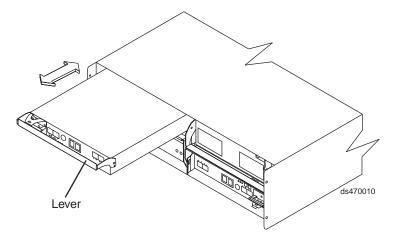
Figure 71. Removing a controller from the DS4200 Express
