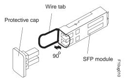
Figure 70. Unlocking the SFP module latch - wire variety
