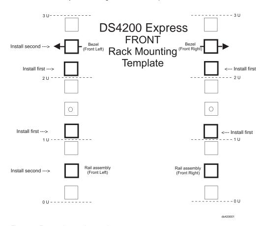
Figure 82. Front rack mounting template
