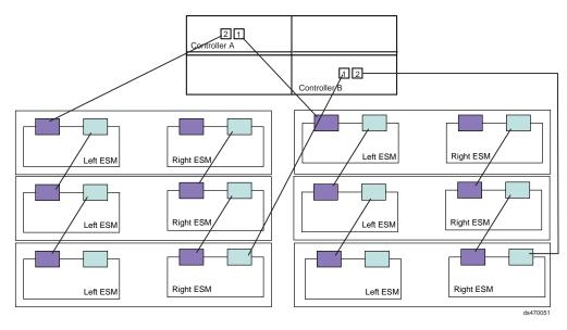
Figure 44. One DS4200 Express and up to six storage expansion enclosure — Recommended cabling
