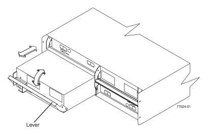
Figure 20. Replacing a power supply and fan unit
