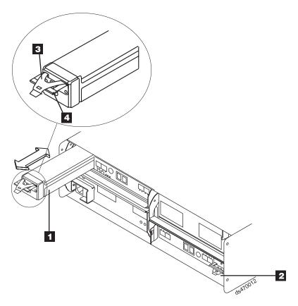
Figure 78. Removing and replacing a battery unit from the controller chassis
