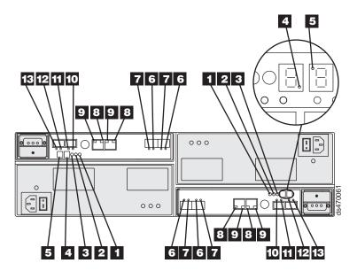
Figure 65. Rear controller LEDs, controls, and connectors
