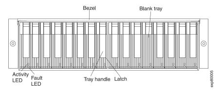
Figure 73. Hot-swap hard disk drive LEDs
