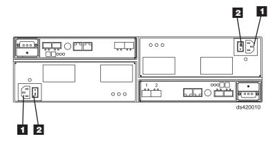
Figure 61. Power supply switches and connectors for the DS4200 Express
