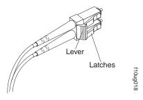
Figure 35. LC-LC fibre-channel cable lever and latches
