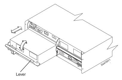
Figure 15. Removing a power supply and fan unit
