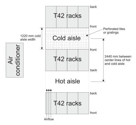
Figure 9. Example of cold aisle/hot aisle rack configuration
