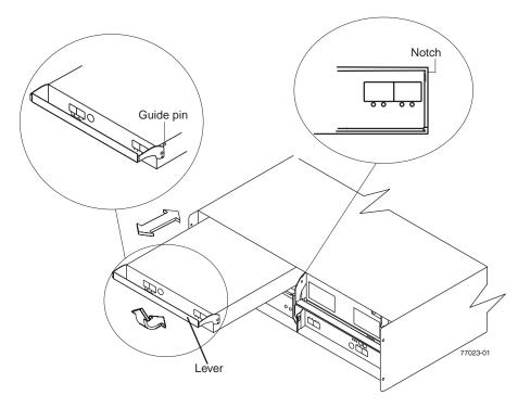
Figure 72. Installing a controller
