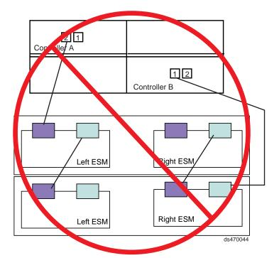
Figure 40. One DS4200 Express and two storage expansion enclosure — Not recommended cabling
