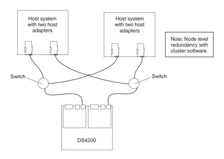
Figure 58. Example of a dual SAN fabric configuration
