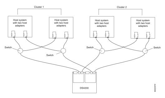
Figure 60. Example of a two-cluster configuration
