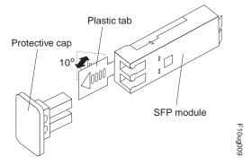
Figure 69. Unlocking the SFP module latch - plastic variety
