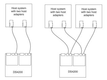
Figure 56. Examples of redundant host direct attached fibre channel configurations
