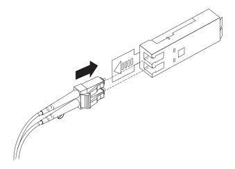
Figure 29. Inserting an LC-LC fibre-channel cable into an SFP module
