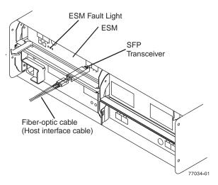
Figure 79. Replacing an SFP module
