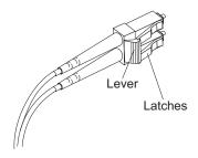
Figure 30. LC-LC fibre-channel cable lever and latches
