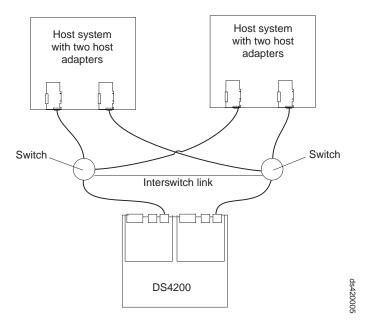
Figure 57. Example of a single SAN fabric configuration
