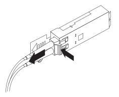
Figure 31. Removing the LC-LC fibre-channel cable
