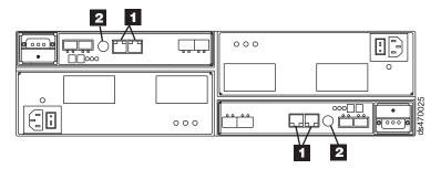
Figure 51. Ethernet and serial port locations on the DS4200 Express
