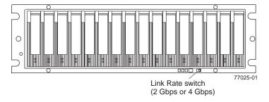
Figure 76. Link rate switch
