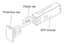
Figure 23. SFP module and protective cap
