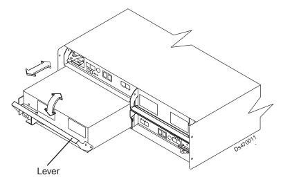
Figure 77. Replacing a power supply and fan unit
