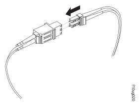
Figure 34. Connecting an LC-LC cable into the LC-SC cable adapter
