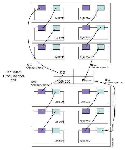
Figure 37. Example of a redundant drive channel pair
