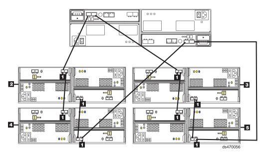
Figure 49. One DS4200 Express and four EXP420 storage expansion enclosures behind a pair of DS4200 Express drive ports
