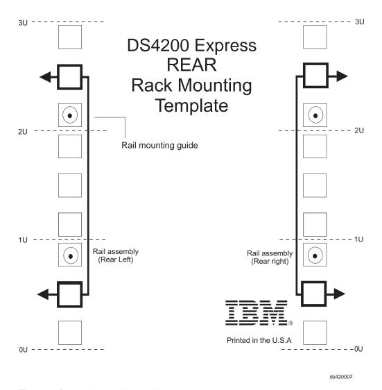
Figure 83. Rear rack mounting template
