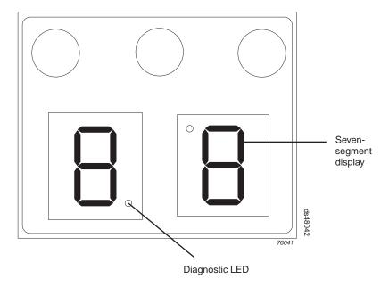
Figure 66. Numeric display LEDs
