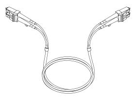
Figure 27. LC-LC fibre-channel cable
