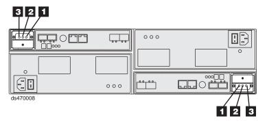
Figure 68. Battery unit LEDs
