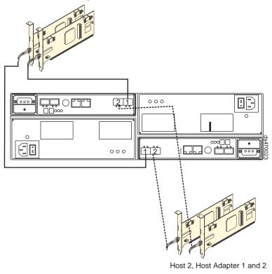
Figure 55. Cabling diagram for two redundant host connections
