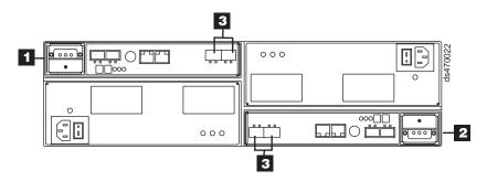
Figure 54. Location of host cables on RAID controllers on the DS4200 Express
