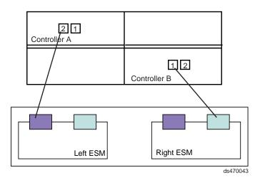
Figure 39. One DS4200 Express and one storage expansion enclosure — Recommended cabling
