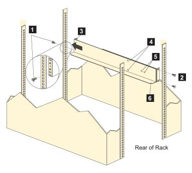
Figure 13. Installing the support rails
