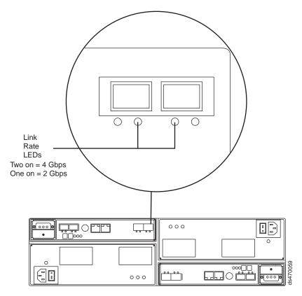
Figure 75. Link rate LEDs
