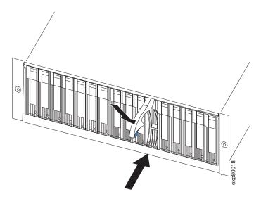
Figure 21. Replacing an EV-DDM
