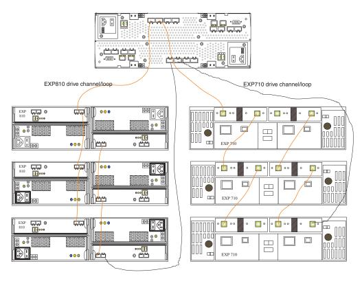
Figure 9. Preferred intermixed DS4000 EXP710 and EXP810 loop configuration
