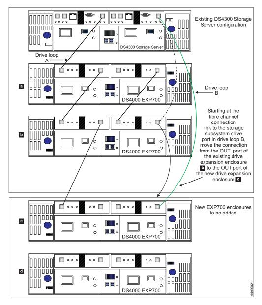
Figure 38. Cabling a single drive enclosure to the end of a functioning drive loop (step 2 of 3)
