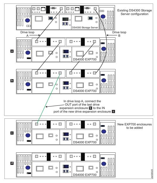
Figure 37. Cabling a single drive enclosure to the end of a functioning drive loop (step 1 of 3)
