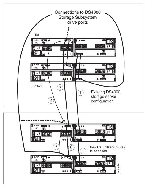
Figure 36. Cabling a second EXP810 drive enclosure to the top of a functioning drive loop
