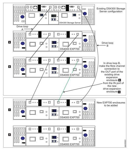
Figure 39. Cabling a single drive enclosure to the end of a functioning drive loop (step 3 of 3)
