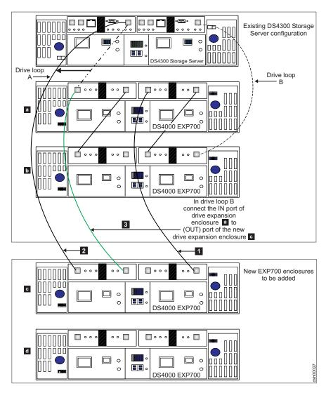
Figure 42. Cabling a single drive enclosure to the beginning of a functioning drive loop (step 3 of 3)
