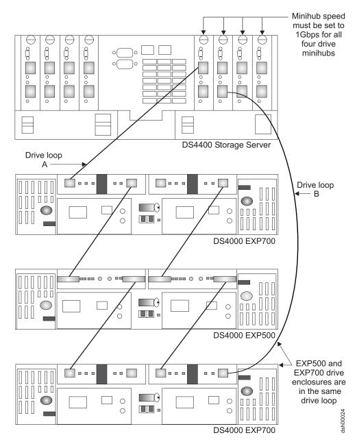
Figure 1. DS4000 EXP500 and EXP700 cabling in a mixed configuration
