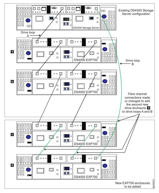
Figure 32. Cabling a second drive enclosure to the end of a functioning drive loop
