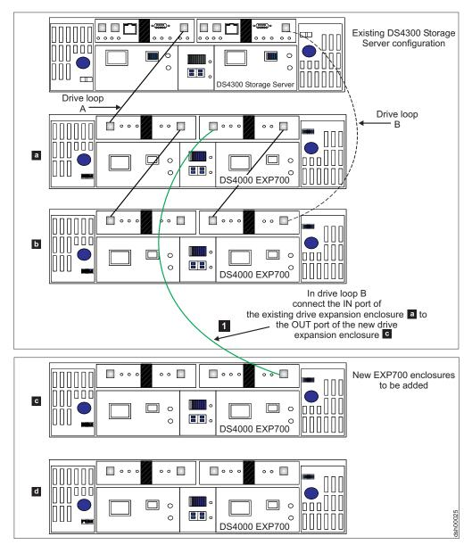
Figure 40. Cabling a single drive enclosure to the beginning of a functioning drive loop (step 1 of 3)
