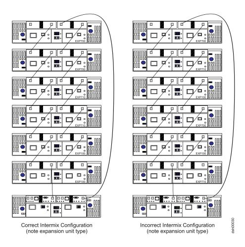
Figure 10. Correct and incorrect ways to group DS4000 storage expansion enclosures in a redundant drive loop
