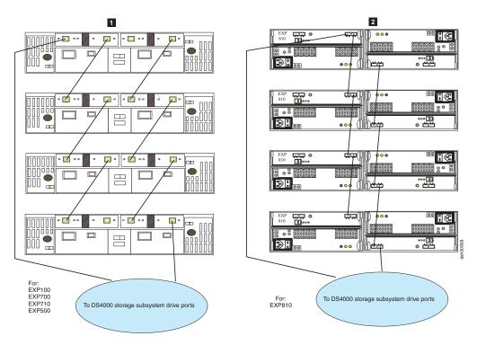
Figure 11. Recommended cable loop scheme for connecting DS4000 storage devices
