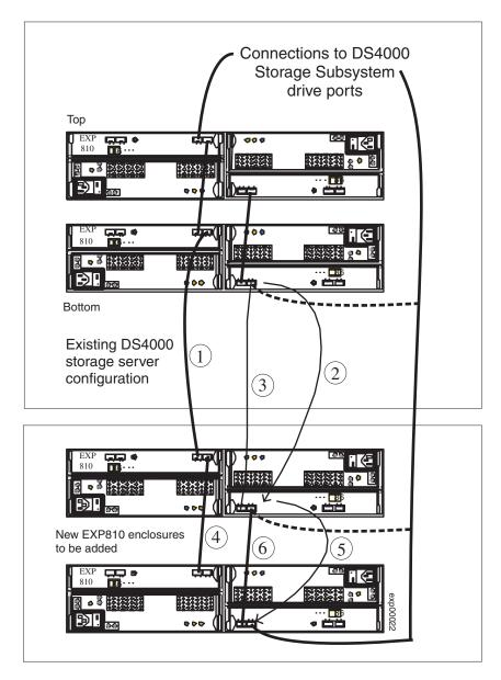
Figure 35. Cabling a second EXP810 drive enclosure to the end of a functioning drive loop
