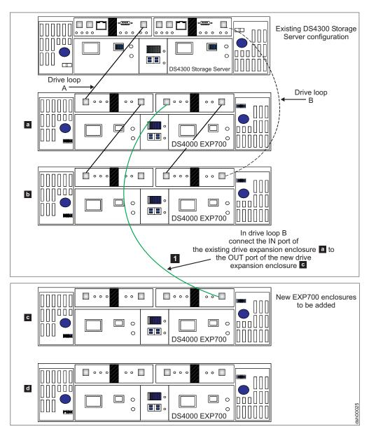
Figure 28. Cabling a single drive enclosure to the beginning of a functioning drive loop (step 1 of 3)
