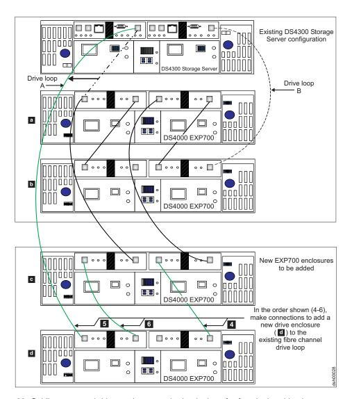
Figure 33. Cabling a second drive enclosure to the beginning of a functioning drive loop
