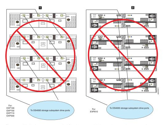
Figure 12. Method **not** recommended for alternate cable loop scheme, when connecting DS4000 storage devices
