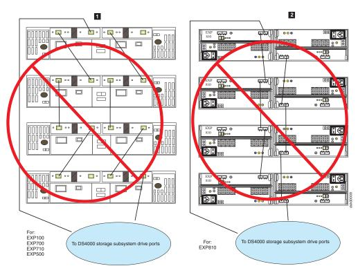
Figure 15. Unacceptable cable loop scheme for connecting DS4000 storage devices
