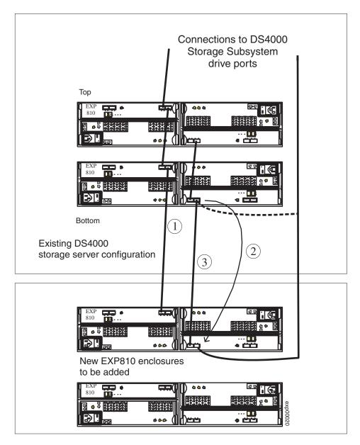
Figure 27. Cabling an EXP810 to the end of a functioning drive loop
