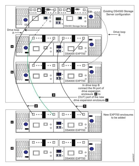
Figure 30. Cabling a single drive enclosure to the beginning of a functioning drive loop (step 3 of 3)
