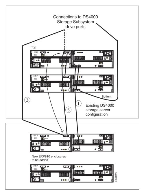
Figure 31. Cabling an EXP810 to the top of a functioning drive loop
