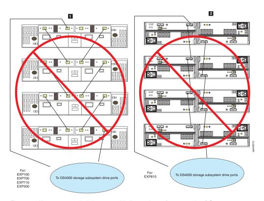
Figure 13. Not recommended alternate cable loop scheme for connecting DS4000 storage devices
