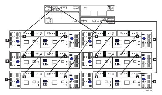
Figure 54. One DS4700 and a maximum of six EXP710 storage expansion enclosures behind a pair of DS4700 drive ports
