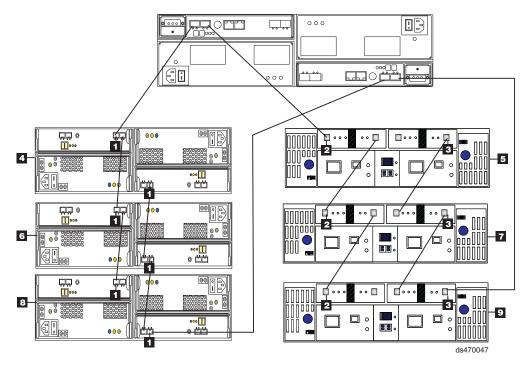
Figure 60. One DS4700 and two or more storage expansion enclosures in a mixed environment — Recommended cabling
