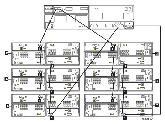
Figure 59. One DS4700 and a maximum of six EXP810 storage expansion enclosures behind a pair of DS4700 drive ports
