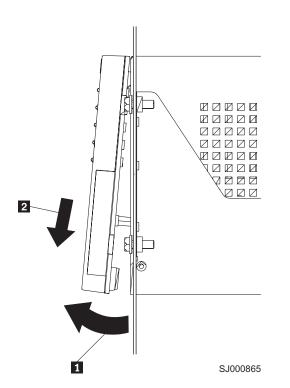
Figure 8. Removing the controller-unit bezel (machine types 3552 [FAStT500] and 1742 [DS4400 and DS4500])
