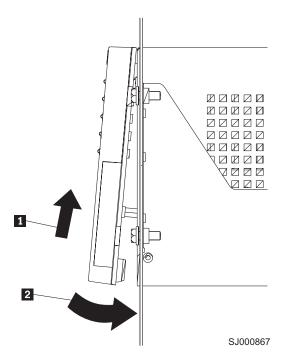
Figure 9. Replacing the controller-unit bezel (machine types 3552 [FAStT500] and 1742 [DS4400 and DS4500])
