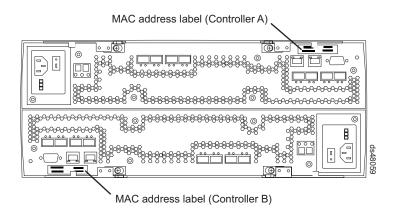
Figure 7. Location of MAC address on DS4800 RAID controllers
