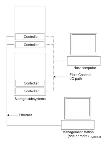
Figure 2. Direct-management (out-of-band) storage subsystems
