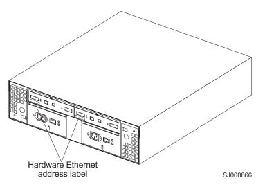
Figure 10. Locating the Ethernet MAC address (machine types 3542 [FAStT200], 1724 [DS4100], and 1722 [DS4300])
