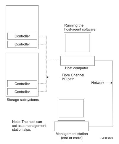
Figure 1. Host-agent (in-band) managed storage subsystems
