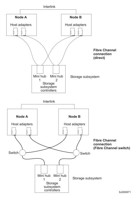
Figure 13. Installing the storage subsystem on a fibre-channel network
