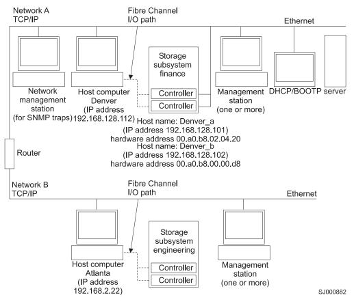
Figure 3. Sample network using directly-managed and host-agent managed storage subsystems
