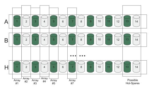
Figure 12. Orthogonally striped RAID arrays - Option 1
