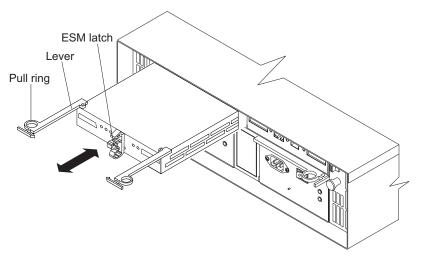
Figure 23. Replacing an ESM
