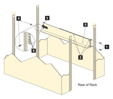
Figure 17. Installing the support rails
