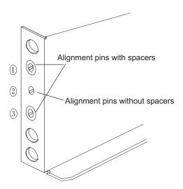
Figure 16. Alignment pins with and without spacers
