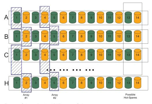
Figure 13. Orthogonally striped RAID arrays - Option 2
