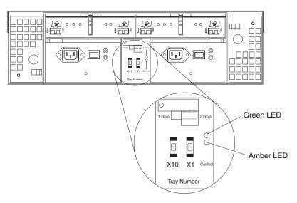
Figure 26. Enclosure ID switches
