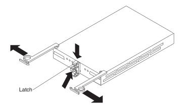
Figure 47. Removing the failed ESM
