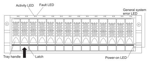
Figure 43. Hot-swap hard disk drive LEDs
