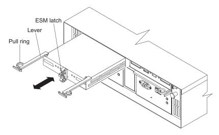
Figure 18. Removing an ESM
