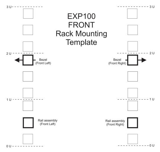
Figure 14. Front rack mounting template
