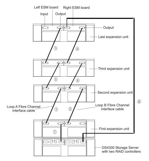
Figure 41. EXP100 redundant loop configuration
