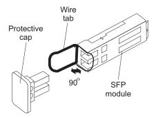
Figure 31. Unlocking the SFP module latch - wire variety
