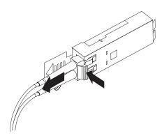
Figure 36. Removing the LC-LC Fibre Channel cable
