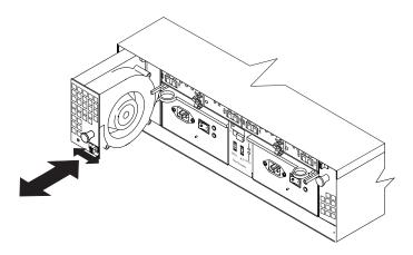
Figure 48. Replacing a hot-swap cooling fan
