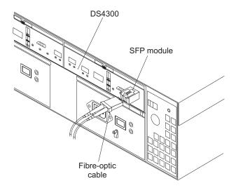
Figure 37. Connecting cables to the installed SFP on a DS4300
