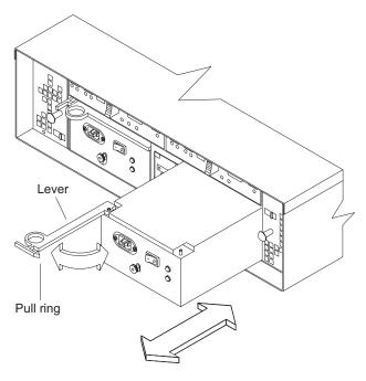
Figure 24. Replacing a power supply
