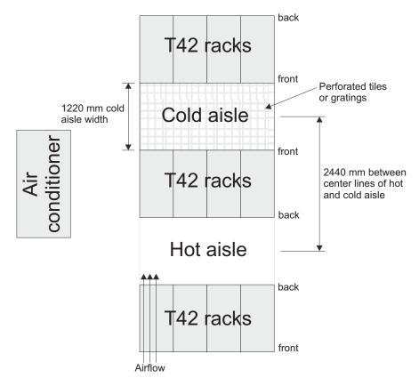
Figure 8. Example of cold aisle/hot aisle rack configuration
