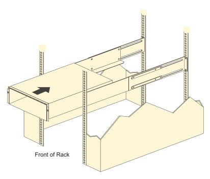
Figure 22. Installing the EXP100
