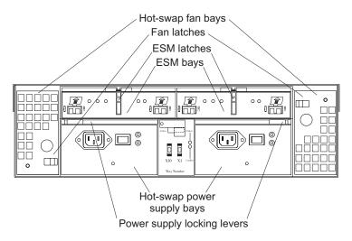
Figure 2. Hot-swap fan, ESM, and power supply bays
