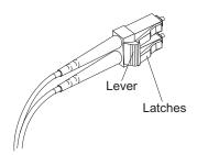
Figure 35. LC-LC Fibre Channel cable lever and latches
