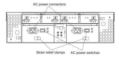
Figure 46. Connecting the power supply
