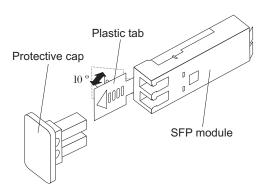
Figure 30. Unlocking the SFP module latch - plastic variety
