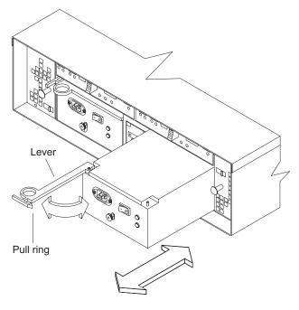
Figure 19. Removing a power supply
