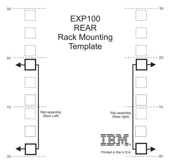
Figure 51. Rear rack mounting template
