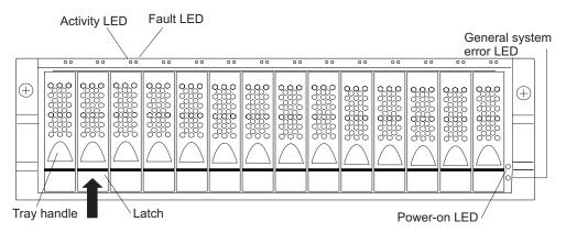
Figure 3. Front controls and indicators
