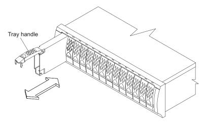
Figure 21. Removing a drive CRU
