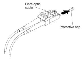
Figure 33. Removing fiber-optic cable protective caps
