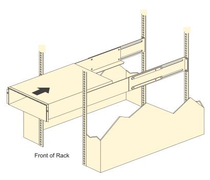
Figure 17. Installing the EXP100
