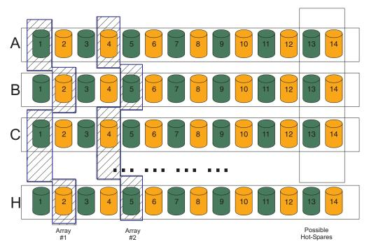
Figure 50. Orthogonally striped RAID arrays - Option 2
