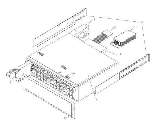
Figure 44. EXP100 storage expansion unit parts list
