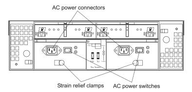
Figure 41. Connecting the power supply
