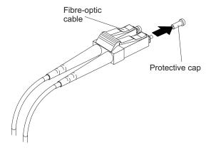
Figure 28. Removing fiber-optic cable protective caps
