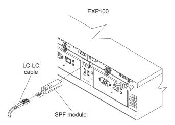
Figure 33. Installing an SFP module and connecting an LC-LC cable to the EXP100
