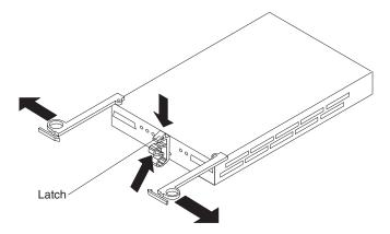
Figure 42. Removing the failed ESM
