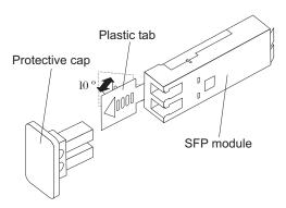
Figure 25. Unlocking the SFP module latch - plastic variety
