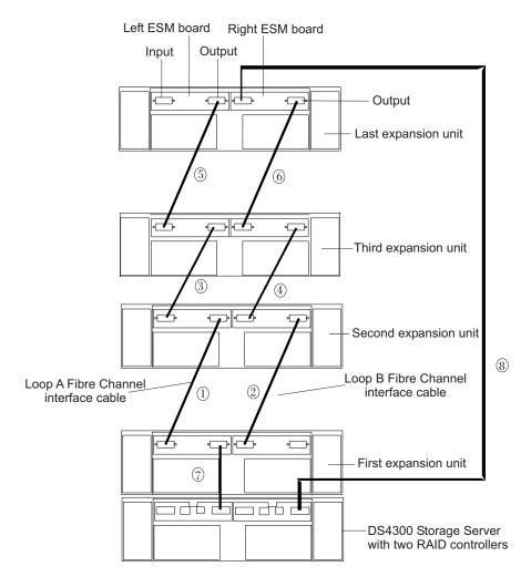
Figure 36. EXP100 redundant loop configuration
