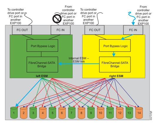
Figure 47. The right ESM and controller firmware recover from a loss of connectivity to the input port of the left ESM
