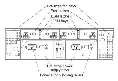
Figure 3. Hot-swap fan, ESM, and power supply bays
