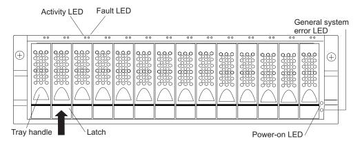
Figure 4. Front controls and indicators
