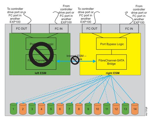
Figure 48. Right ESM reroutes I/Os along dashed alternate paths
