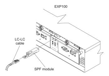
Figure 35. Installing an SFP module and connecting an LC-LC cable to the EXP100
