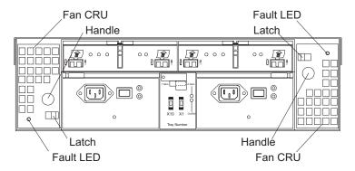
Figure 6. Fan controls and indicators
