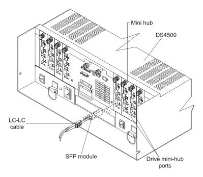
Figure 34. Installing an SFP module and LC-LC cable in a DS4500
