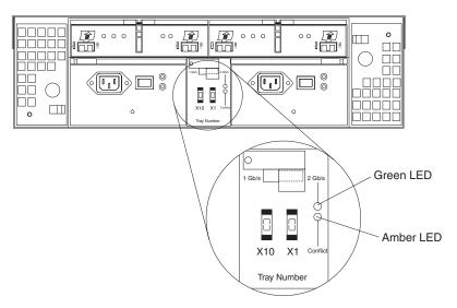
Figure 21. Enclosure ID switches
