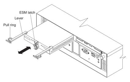
Figure 13. Removing an ESM
