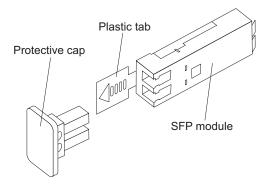
Figure 23. SFP module and protective cap
