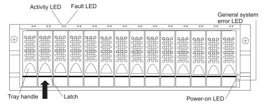
Figure 38. Hot-swap hard disk drive LEDs
