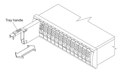
Figure 16. Removing a drive CRU
