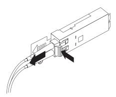
Figure 31. Removing the LC-LC fibre-channel cable
