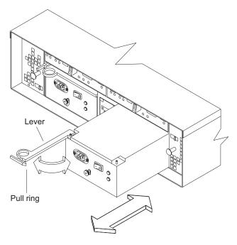
Figure 14. Removing a power supply
