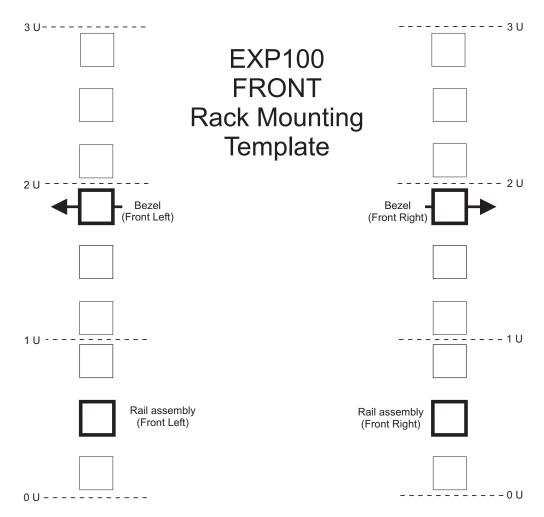
Figure 9. Front rack mounting template
