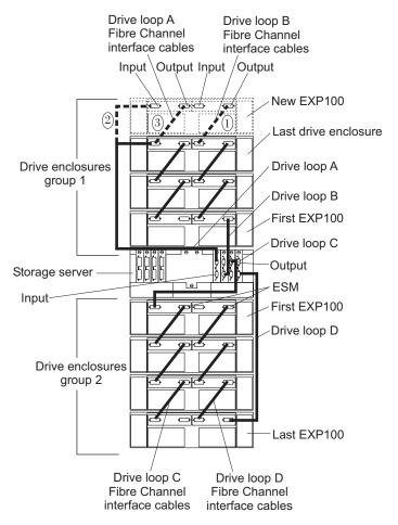
Figure 37. Cabling the EXP100 to two redundant loops
