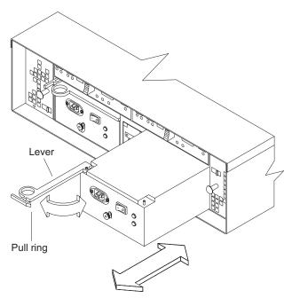
Figure 19. Replacing a power supply
