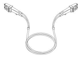
Figure 27. LC-LC fibre-channel cable
