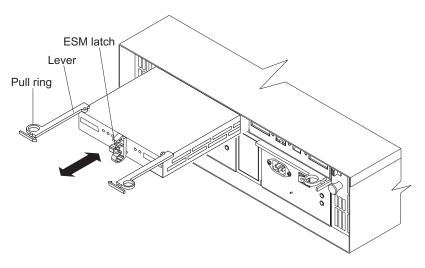
Figure 18. Replacing an ESM
