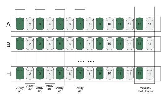
Figure 49. Orthogonally striped RAID arrays - Option 1
