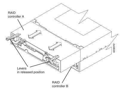
Figure 19. Removing the controllers
