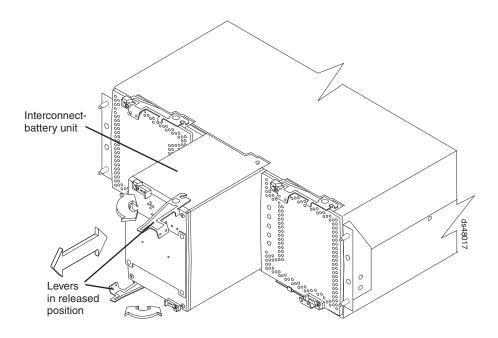
Figure 83. Removing an interconnect-battery unit from the DS4800
