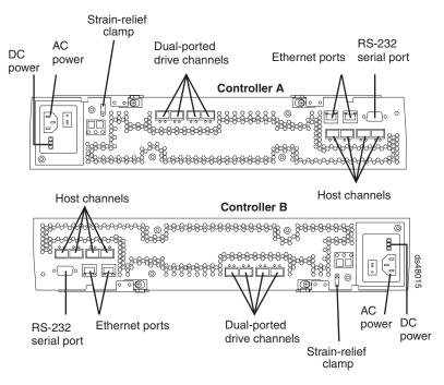
Figure 67. RAID controller connections
