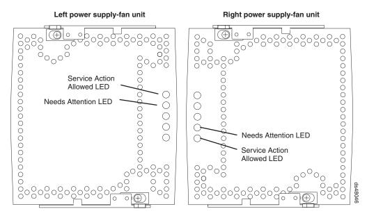
Figure 79. Power supply-fan LEDs
