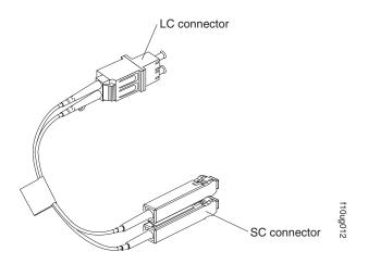
Figure 36. LC-SC fibre-channel cable adapter
