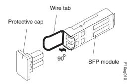
Figure 76. Unlocking the SFP module latch - wire variety
