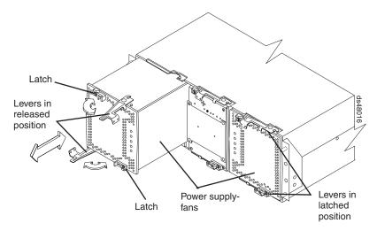
Figure 6. Power supply-fan
