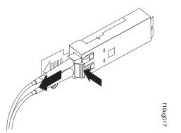
Figure 35. Removing the LC-LC fibre-channel cable
