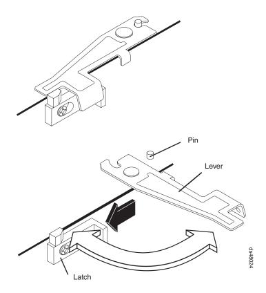
Figure 16. Component lever and latch
