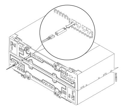
Figure 88. Replacing an SFP module
