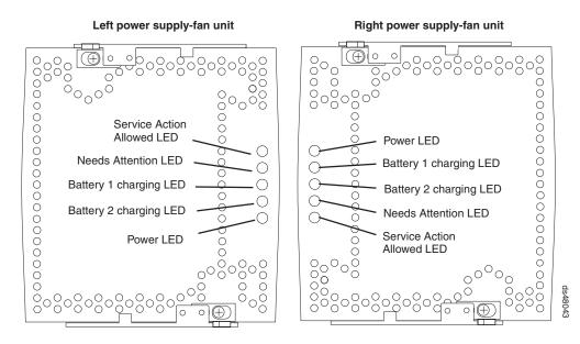
Figure 64. Power supply-fan LEDs
