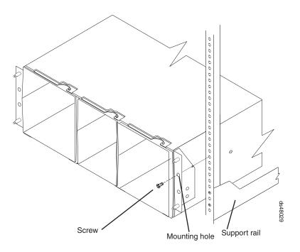
Figure 20. Securing the DS4800 to the rack cabinet
