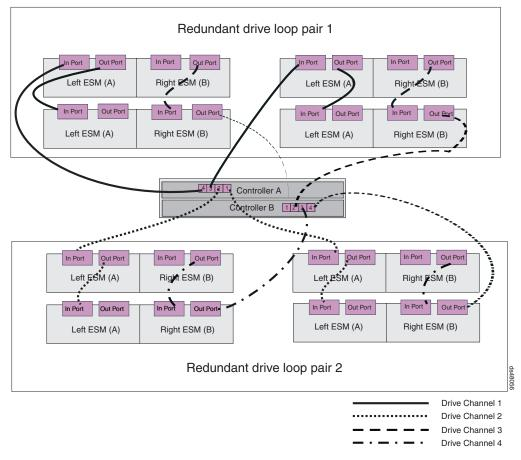
Figure 42. Example 2 of redundant drive loop pairs
