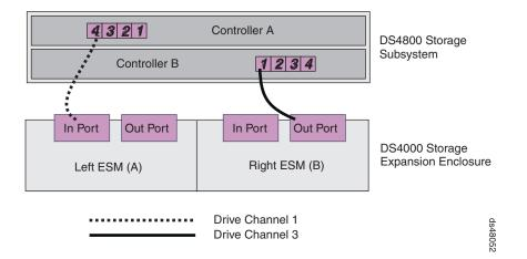
Figure 44. One DS4800 and one storage expansion enclosure — Recommended cabling
