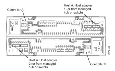
Figure 48. Location of host cables on RAID controllers
