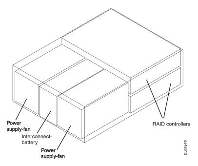
Figure 3. Location of components in the storage subsystem
