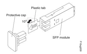
Figure 75. Unlocking the SFP module latch - plastic variety
