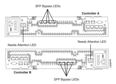
Figure 87. Needs Attention and SFP Model Bypass LEDs
