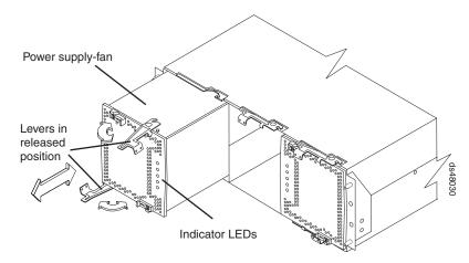
Figure 21. Replacing the power supply-fans
