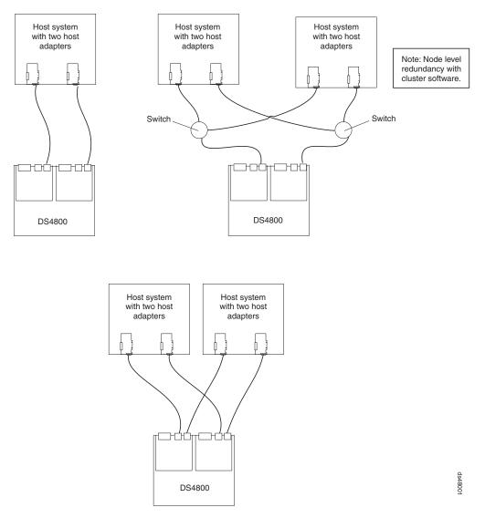
Figure 53. Examples of redundant host and drive fibre channel loop configurations
