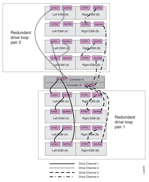
Figure 41. Example 1 of redundant drive loop pairs
