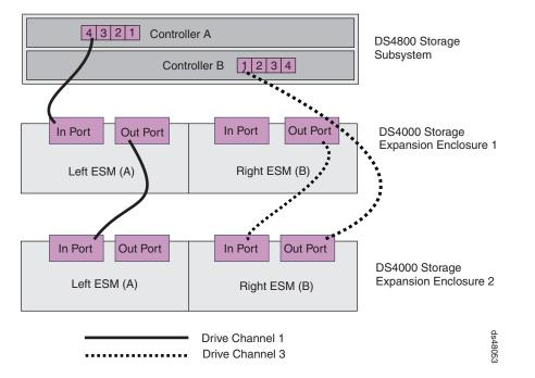
Figure 45. One DS4800 and two storage expansion enclosures — Recommended cabling
