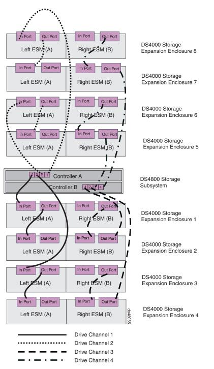
Figure 47. One DS4800 and eight storage expansion enclosures — Recommended cabling
