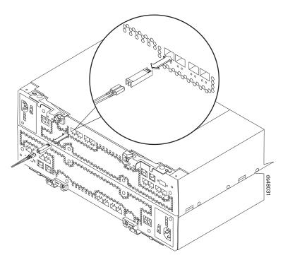
Figure 26. Replacing an SFP module
