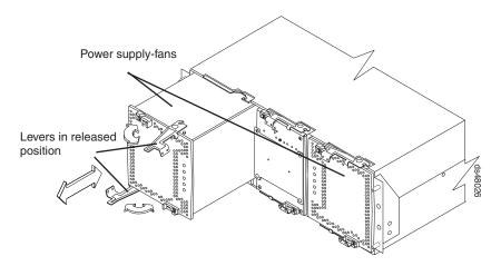
Figure 17. Removing the power supply-fans
