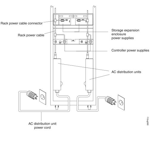
Figure 58. Redundant AC power connections to controllers and storage expansion enclosures
