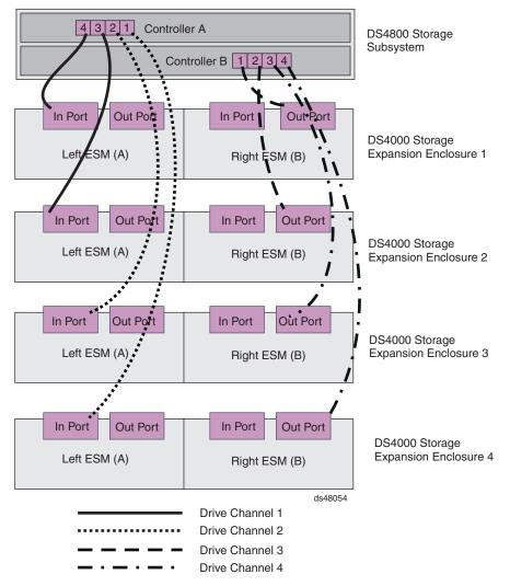
Figure 46. One DS4800 and four storage expansion enclosures — Recommended cabling
