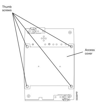
Figure 85. Battery access cover on the interconnect-battery unit
