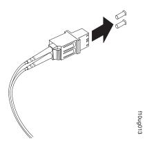
Figure 37. Removing the LC-SC cable adapter protective caps
