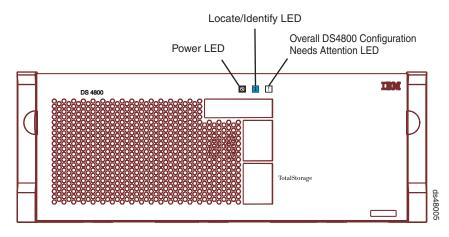
Figure 84. Overall DS4800 Configuration Needs Attention LED on the DS4800 front bezel
