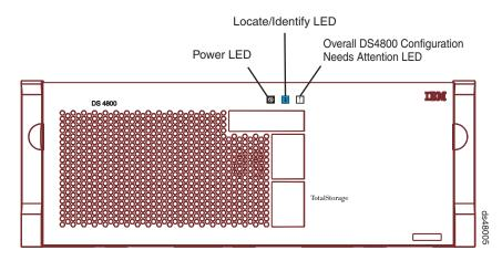
Figure 61. Front bezel LEDs
