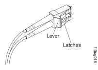
Figure 34. LC-LC fibre-channel cable lever and latches
