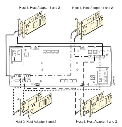
Figure 49. Cabling diagram for four redundant host connections
