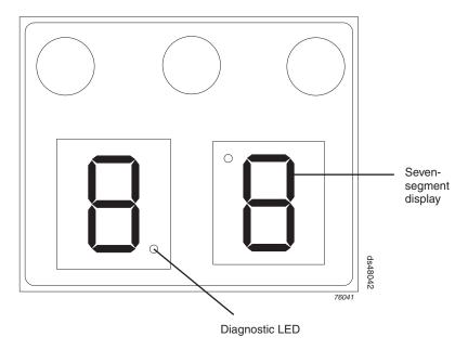
Figure 63. Numeric display LEDs
