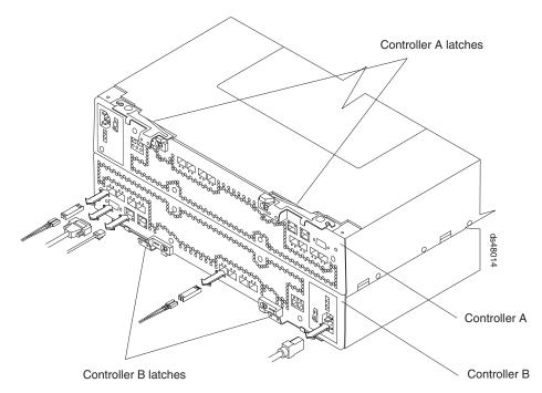
Figure 4. Controllers in the storage subsystem
