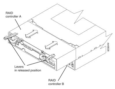
Figure 23. Replacing the controllers
