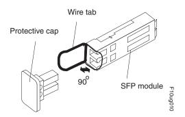
Figure 28. Unlocking the SFP module latch - wire variety
