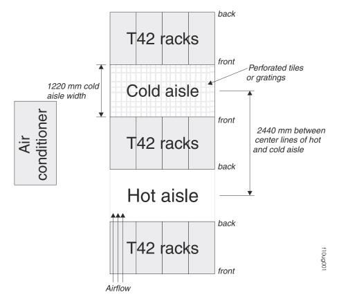
Figure 11. Example of cold aisle/hot aisle rack cabinet configuration
