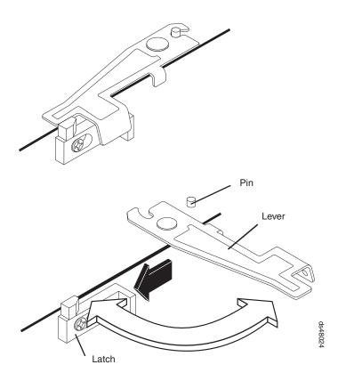
Figure 72. Component lever and latch
