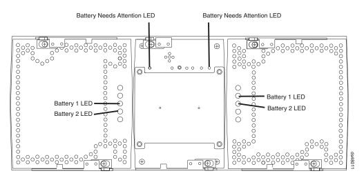
Figure 71. Battery LEDs
