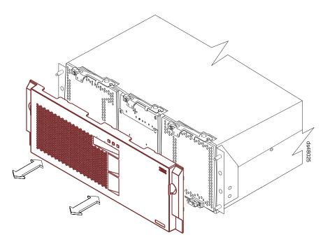
Figure 24. Removing the front bezel
