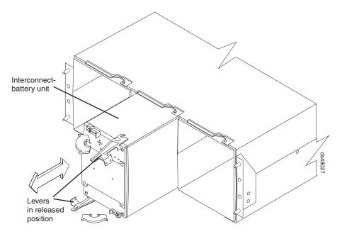
Figure 18. Removing the interconnect-battery unit
