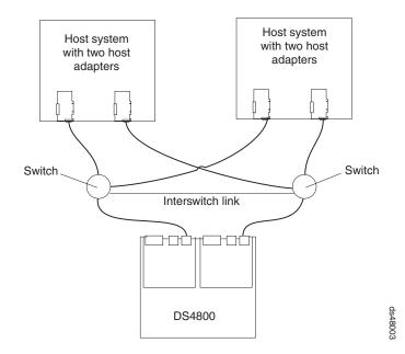
Figure 54. Example of a single SAN fabric configuration
