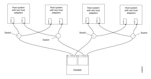
Figure 56. Example of a two-cluster configuration
