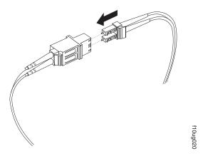
Figure 38. Connecting an LC-LC cable into the LC-SC cable adapter
