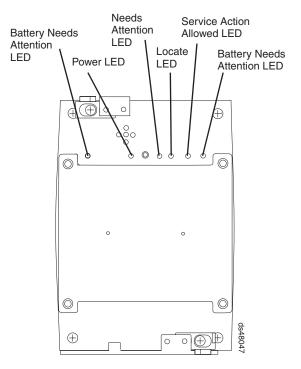
Figure 65. Interconnect-battery unit LEDs
