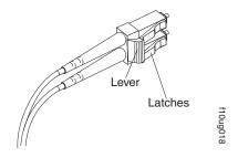
Figure 39. LC-LC fibre-channel cable lever and latches
