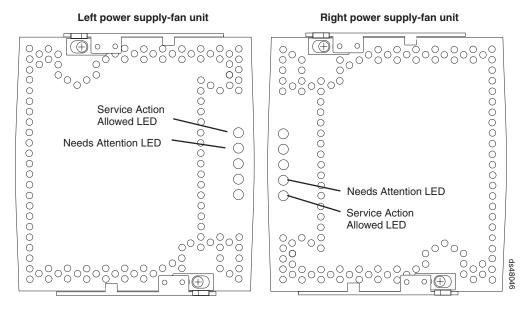
Figure 66. Power supply-fan Needs Attention LEDs
