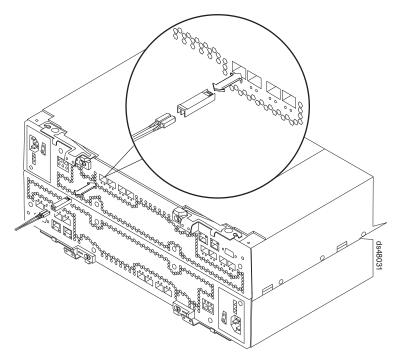
Figure 30. Replacing an SFP module
