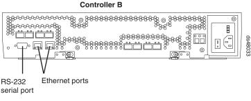
Figure 50. Ethernet and serial port locations
