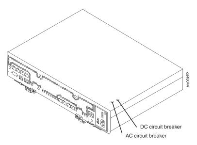
Figure 69. Circuit breaker access holes
