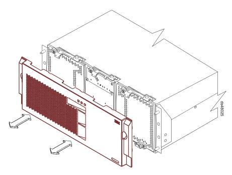
Figure 59. Installing the front bezel
