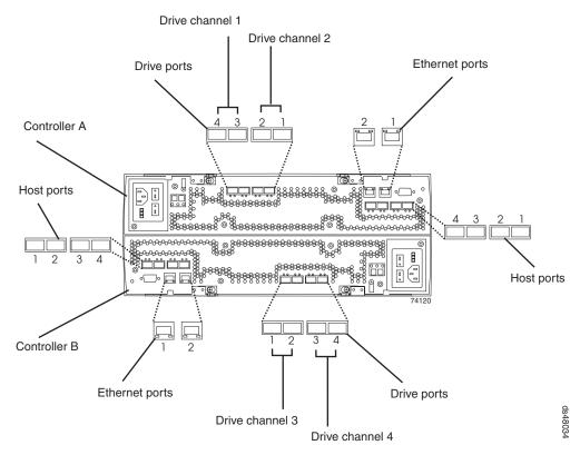
Figure 43. DS4800 Storage Subsystem ports and controllers
