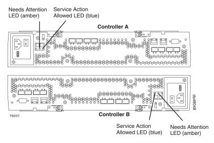
Figure 73. RAID controller Needs Attention and Service Action Allowed LEDs
