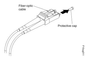
Figure 32. Removing fiber-optic cable protective caps
