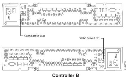
Figure 70. Cache Active LEDs
