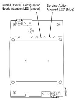
Figure 82. Interconnect-battery unit Needs Attention and Service Action Allowed LEDs
