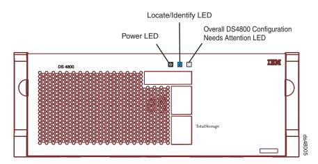
Figure 86. Overall DS4800 Configuration Needs Attention LED on the DS4800 front bezel
