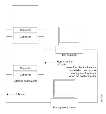
Figure 52. Direct (out-of-band) managed storage subsystems
