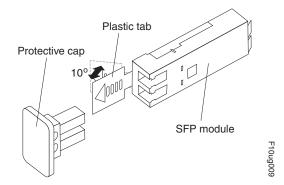
Figure 27. Unlocking the SFP module latch - plastic variety
