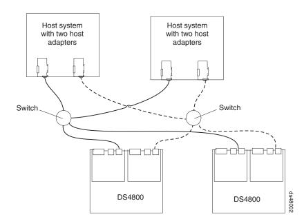
Figure 55. Example of a dual SAN fabric configuration
