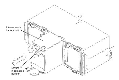
Figure 22. Replacing the interconnect-battery unit
