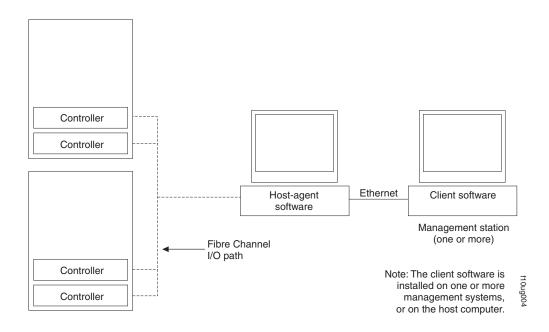
Figure 51. Host-agent (in-band) managed storage subsystems
