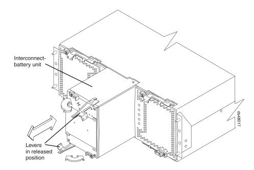
Figure 7. Interconnect-battery unit
