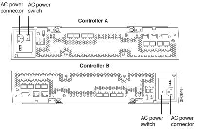
Figure 60. AC power switches on the controllers
