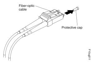
Figure 29. Removing caps from fiber-optic cables
