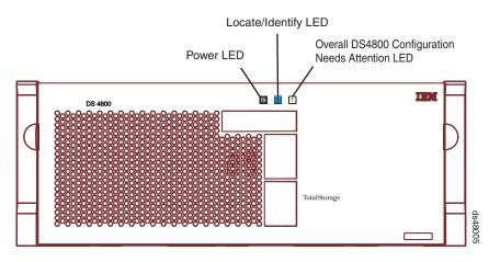
Figure 78. Overall DS4800 Configuration Needs Attention LED on the DS4800 front bezel
