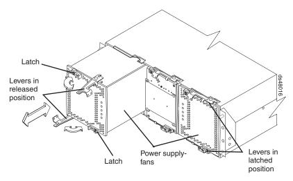
Figure 80. Removing a power supply-fan from the DS4800
