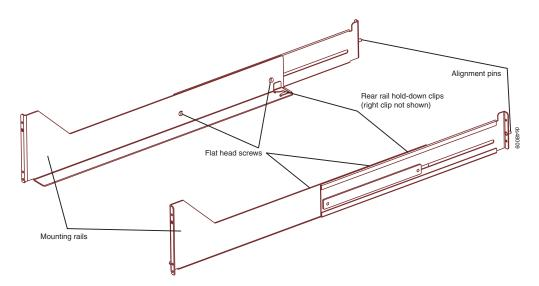
Figure 14. DS4800 support rail assembly
