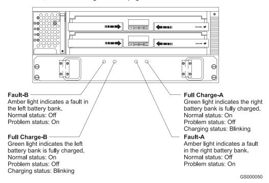
Figure 26. Battery indicator lights
