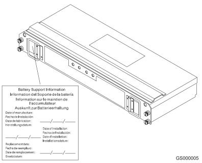
Figure 32. Checking the battery service date
