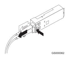
Figure 11. Removing the LC-LC Fibre Channel cable
