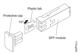
Figure 47. Unlocking the SFP module latch - plastic variety
