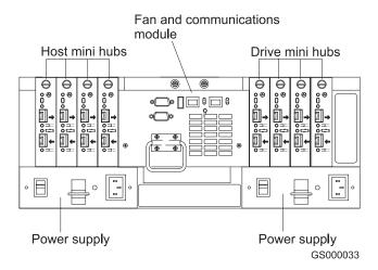
Figure 4. IBM TotalStorage DS4500 Fibre Channel Storage Server - back view
