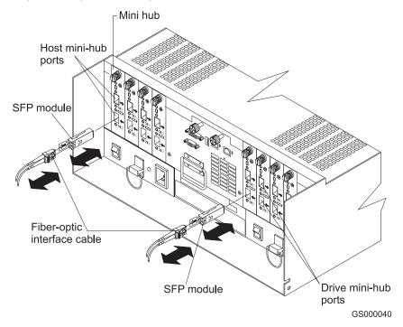
Figure 46. Replacing a failed SFP module
