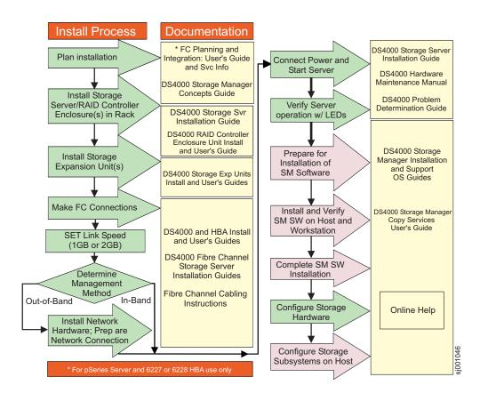
Figure 1. Installation process flow by current publications
