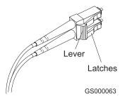
Figure 10. LC-LC Fibre Channel Cable lever and latches
