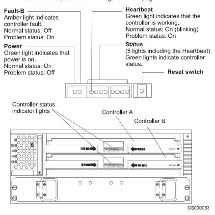
Figure 25. RAID controller indicator lights
