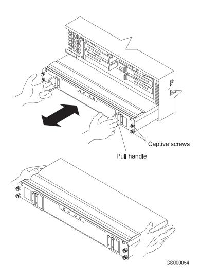
Figure 36. Removing and installing a battery
