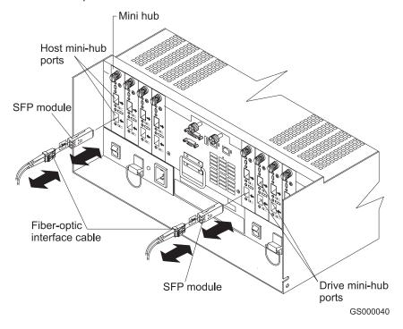
Figure 5. Fibre Channel interface connections
