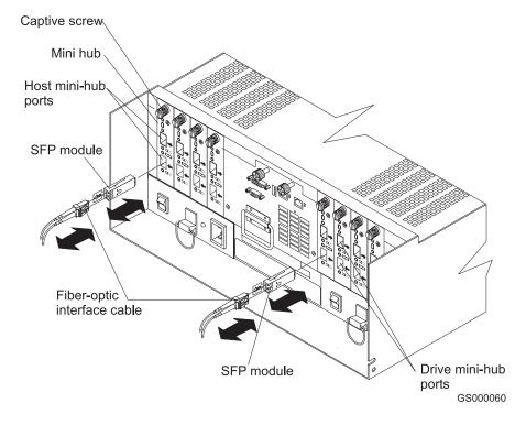
Figure 51. Removing the fiber-optic cable from the SFP module
