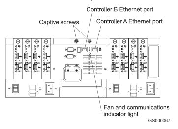
Figure 42. Fan and communications module ports and indicator light
