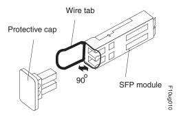
Figure 48. Unlocking the SFP module latch - wire variety
