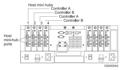
Figure 18. Host-side mini-hub interface ports
