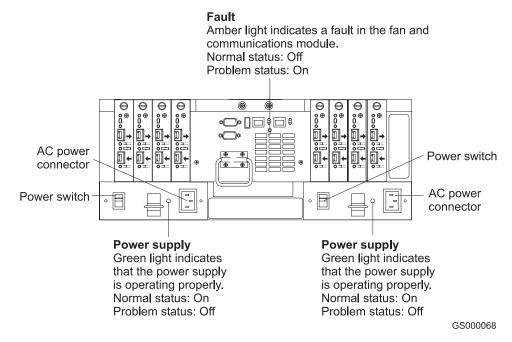
Figure 44. Power supply switch, ac power connectors, and indicator lights
