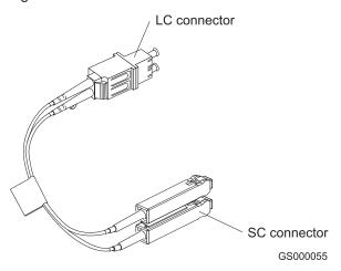
Figure 12. LC-SC Fibre Channel cable
