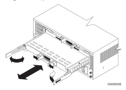
Figure 34. Removing and replacing a failed controller CRU
