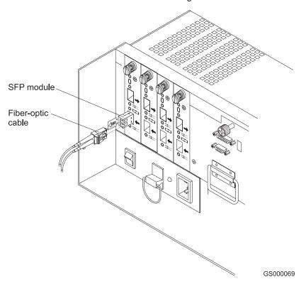
Figure 9. Inserting an LC-LC Fibre Channel cable into an installed SFP module
