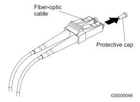
Figure 7. Removing the fiber-optic cable protective caps
