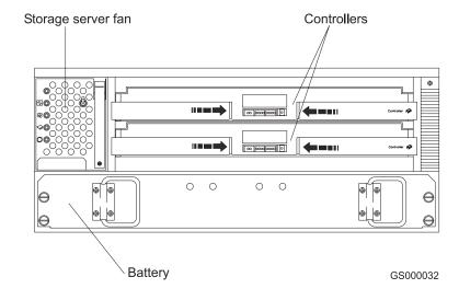
Figure 3. IBM TotalStorage DS4500 Fibre Channel Storage Server front view
