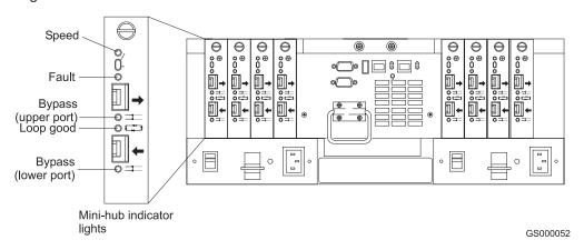
Figure 29. Mini-hub indicator lights
