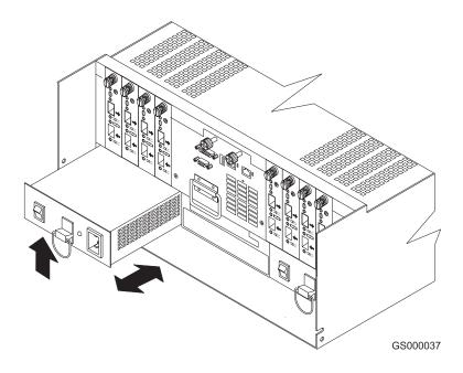
Figure 45. Removing and installing a power supply CRU
