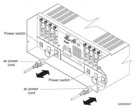
Figure 23. Connecting the power cords and power switch locations
