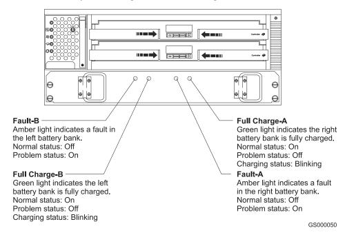
Figure 38. Battery CRU indicator lights
