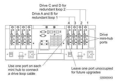
Figure 19. Drive-side mini-hub interface ports
