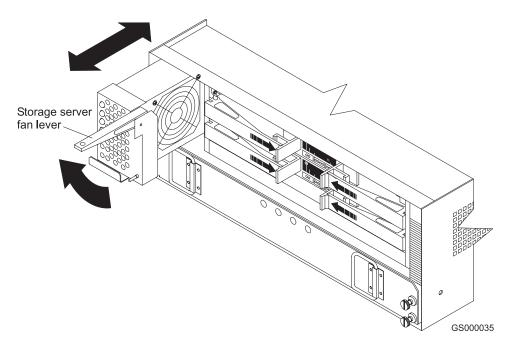
Figure 40. Removing and installing the storage server fan
