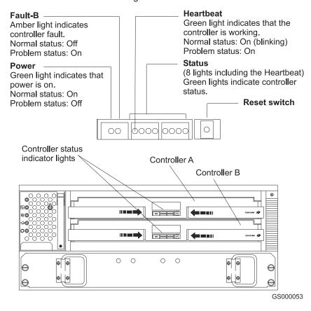
Figure 33. Controller status indicator lights
