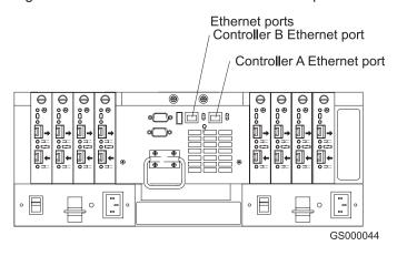
Figure 20. Ethernet interface ports
