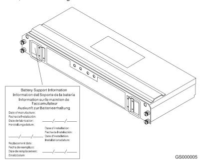
Figure 37. Recording the battery support information
