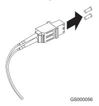
Figure 13. Removing the LC-SC cable adapter protective caps
