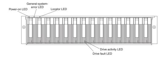
Figure 43. Storage server LEDs (front)
