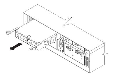
Figure 52. Pull-rings for removing a controller
