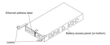
Figure 53. RAID controller levers and labels
