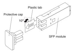
Figure 55. Unlocking the SFP module latch - plastic variety
