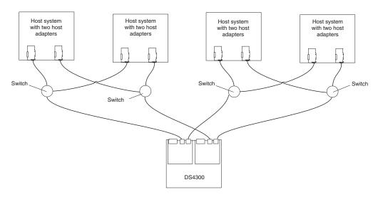
Figure 24. Example of a two-cluster configuration (Model 60U/60X)
