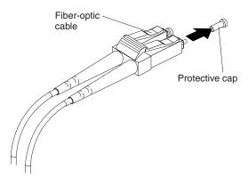
Figure 34. Removing caps from fiber-optic cables
