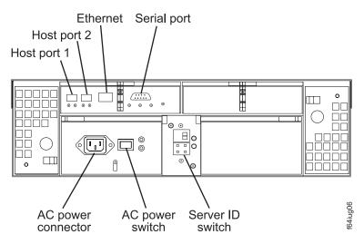
Figure 6. Model 6LU/6LX: Interface ports and switches
