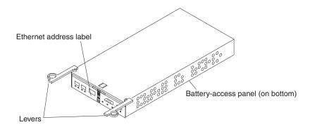
Figure 48. RAID controller levers and labels
