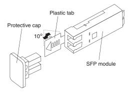
Figure 32. Unlocking the SFP module latch - plastic variety
