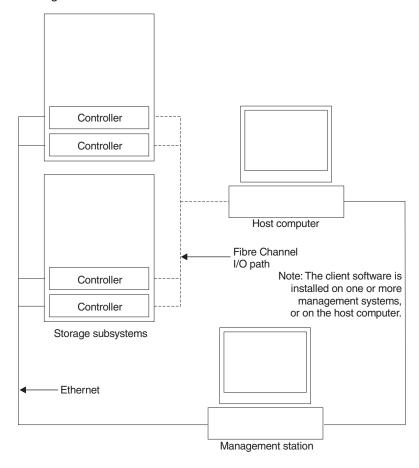
Figure 20. Direct-managed storage subsystems
