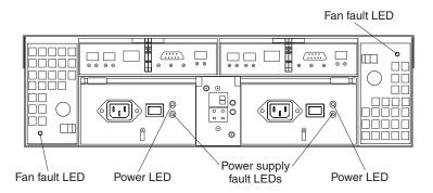
Figure 45. Fan and power supply LEDs
