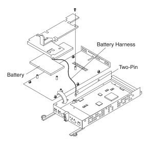
Figure 73. Removing the controller battery
