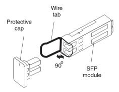
Figure 51. Unlocking the SFP module latch - wire variety
