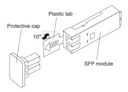
Figure 69. Unlocking the SFP module latch - plastic variety
