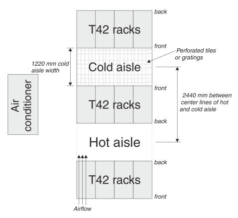
Figure 7. Example of Cold Aisle/Hot Aisle Rack Configuration
