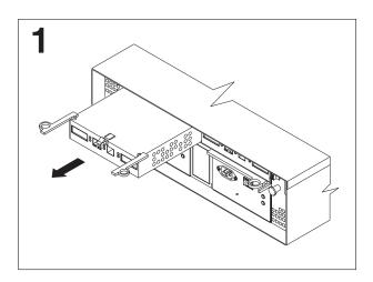
Figure 10. RAID controller removal
