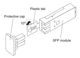
Figure 50. Unlocking the SFP module latch - plastic variety
