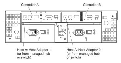
Figure 36. Location of host cables (Model 60U/60X)
