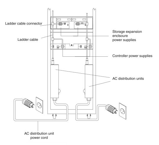
Figure 40. Redundant ac power connections to controllers and storage expansion enclosures
