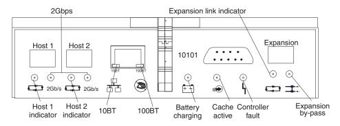
Figure 44. RAID controller LEDs
