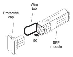
Figure 56. Unlocking the SFP module latch - wire variety
