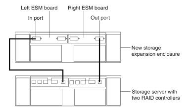
Figure 41. Adding a storage expansion enclosure
