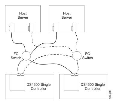
Figure 29. Example of a dual-server, dual-SAN fabric zone configuration with two adapters per server (Model 6LU/6LX)
