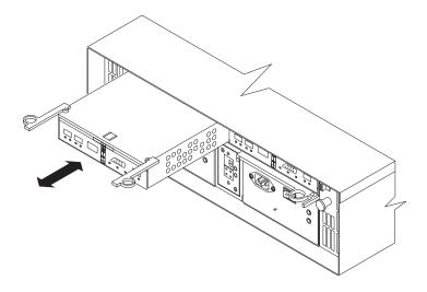
Figure 74. Installing a new RAID controller
