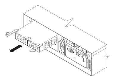
Figure 71. Pull-rings for removing a controller
