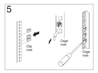
Figure 14. Rack nut installation
