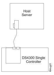
Figure 25. Example of a single server configuration with one adapter (Model 6LU/6LX)
