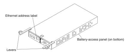
Figure 67. RAID controller levers and labels
