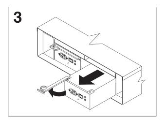
Figure 12. Power supply removal
