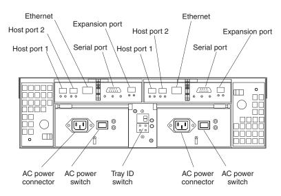
Figure 5. Model 60U/60X: Interface ports and switches
