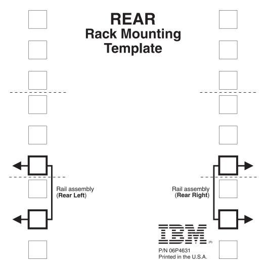
Figure 9. Rear rack mounting template
