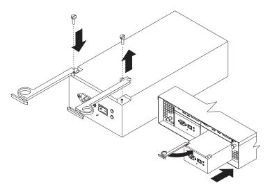
Figure 65. Installing a hot-swap power supply
