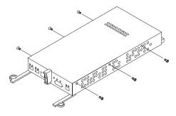
Figure 72. Controller battery-access panel screws
