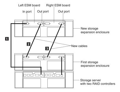
Figure 42. Adding a second storage expansion enclosure
