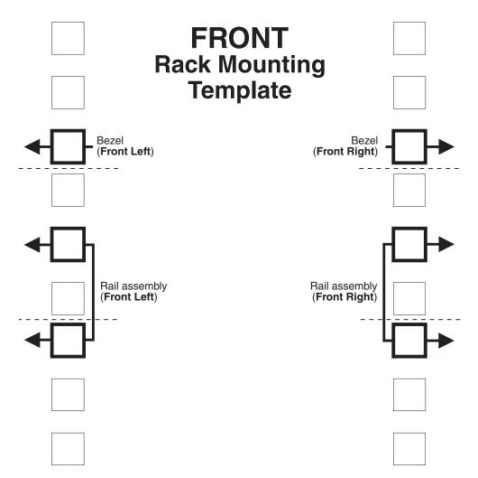
Figure 8. Front rack mounting template
