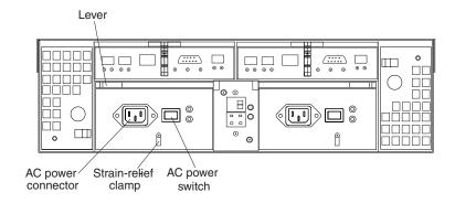
Figure 64. Lever for power supply removal
