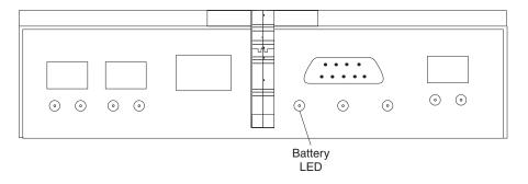
Figure 47. Battery LED
