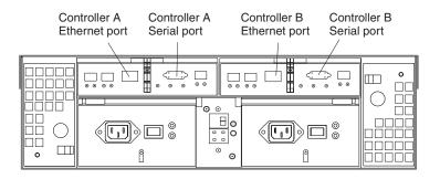
Figure 38. Ethernet and serial port locations
