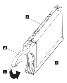
Figure 59. Releasing the drive latch
