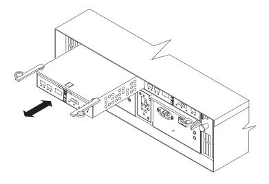
Figure 57. Pull-rings for removing a controller
