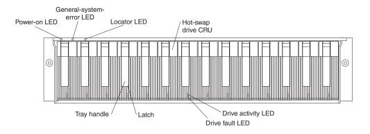
Figure 2. Front controls and components
