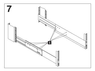
Figure 16. Rail adjustment screws
