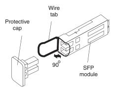
Figure 33. Unlocking the SFP module latch - wire variety
