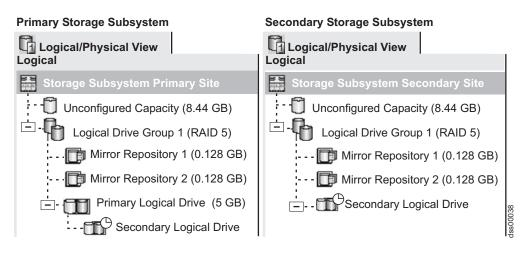
Figure 30. Mirrored logical drive pair showing Synchronization-in-Progress status
