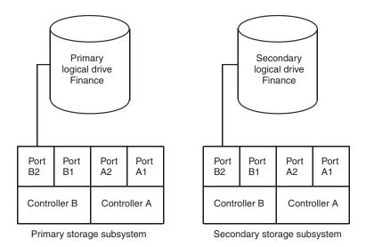
Figure 35. Controller B shown as controller owner
