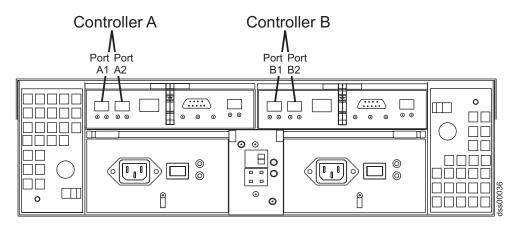
See Figure 32 for the location of controller host ports for machine type 1722.
