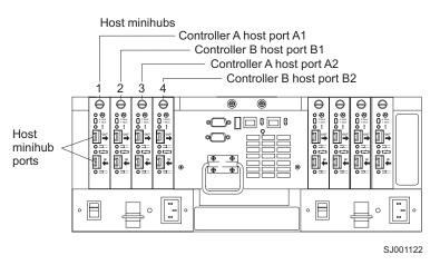
Figure 31. Controller A and Controller B host ports, machine type 3552 and 1742
