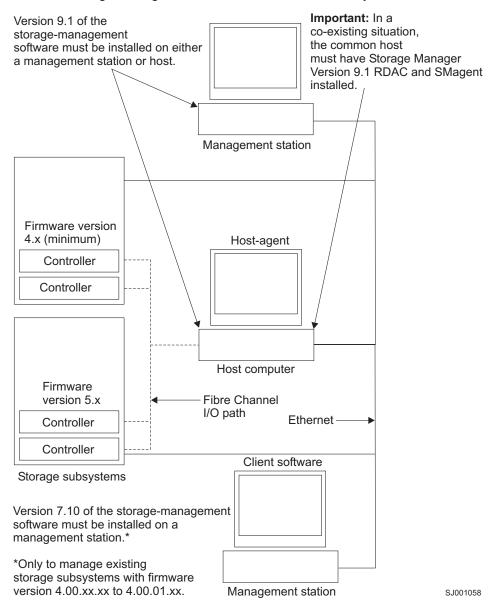
Figure 14. Sample coexisting storage subsystems
