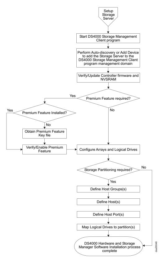
Figure 10. Installation process (part 6 of 6)
