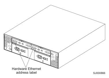
Figure 15. Locating the Ethernet MAC address (machine types 3542 [FAStT200], 1724 [DS4100], and 1722 [DS4300])
