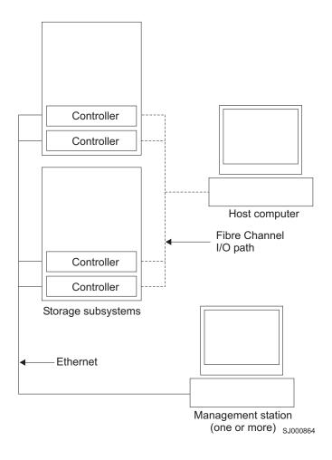
Figure 3. Direct-management (out-of-band) storage subsystems
