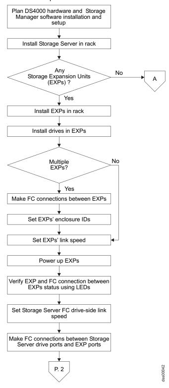
Figure 5. Installation process (part 1 of 6)
