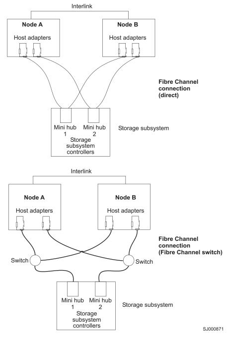
Figure 20. Installing the storage subsystem on a fibre-channel network
