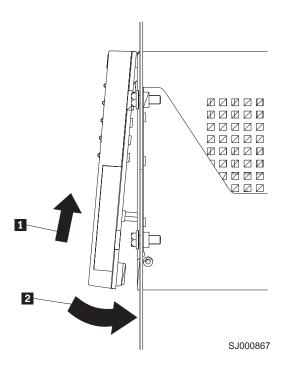
Figure 17. Replacing the controller-unit bezel (machine types 3552 [FAStT500] and 1742 [DS4400 and DS4500])
