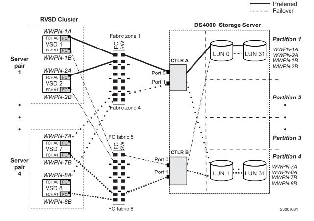
Figure 11. Cluster configuration with single DS4000 storage subsystem — one to four partitions
