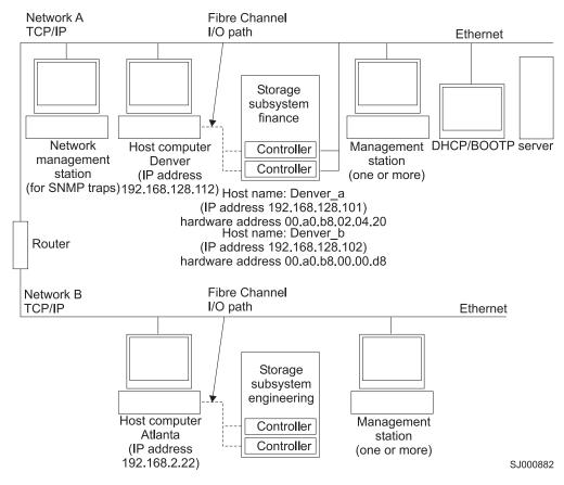
Figure 3. Sample network using both out-of-band and in-band managed storage subsystems
