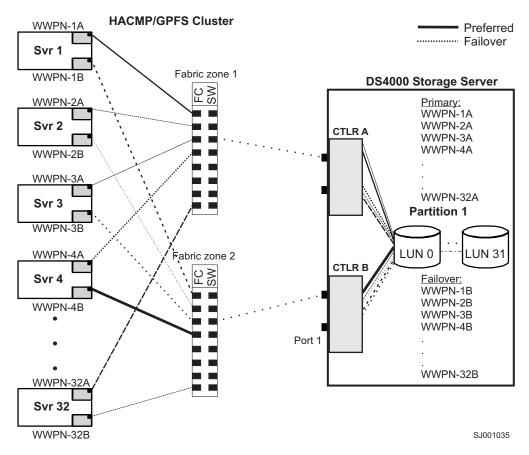
Figure 15. HACMP/GPFS cluster configuration with one DS4000 storage subsystem — one partition
