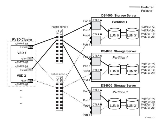
Figure 12. Cluster configuration with three DS4000 storage subsystems — one partition per DS4000
