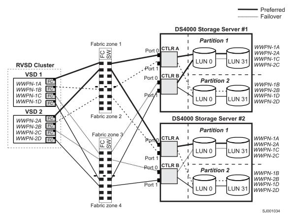
Figure 14. RVSD cluster configuration with two DS4000 storage subsystems — two partitions per DS4000
