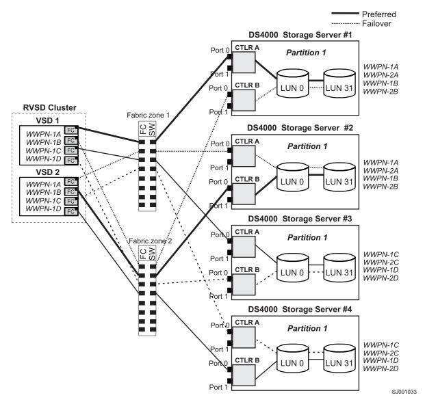
Figure 13. Cluster configuration with four DS4000 storage subsystems — one partition per DS4000
