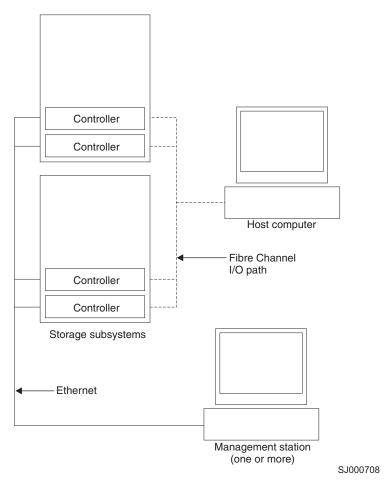
Figure 2. Out-of-band managed storage subsystems
