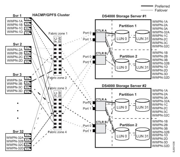
Figure 16. HACMP/GPFS cluster configuration with two DS4000 storage subsystems — two partitions per DS4000
