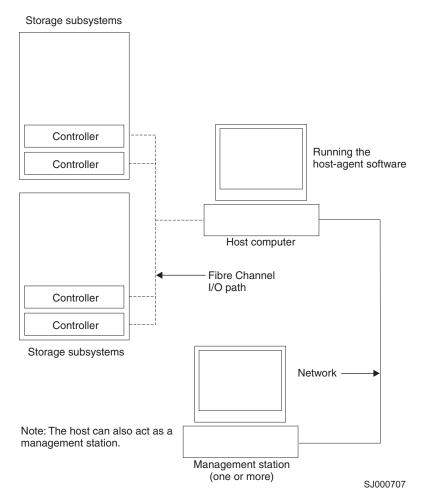
Figure 1. In-band managed storage subsystems
