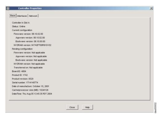
Figure 5. Controller Properties window
