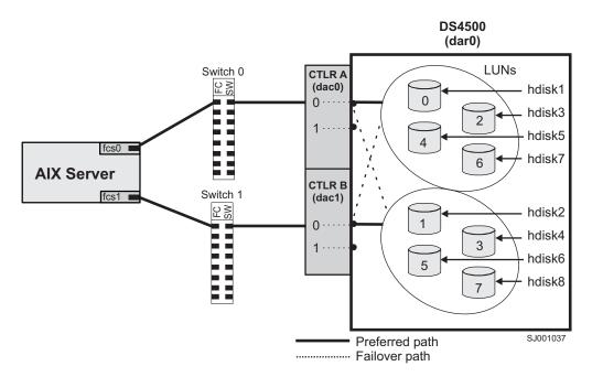
Figure 4. DS4000/AIX system configuration
