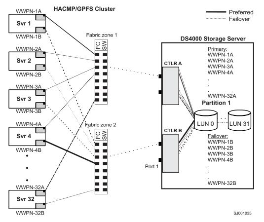
Figure 19. HACMP/GPFS cluster configuration with one DS4000 storage subsystem — one partition
