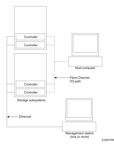
Figure 3. Out-of-band managed storage subsystems
