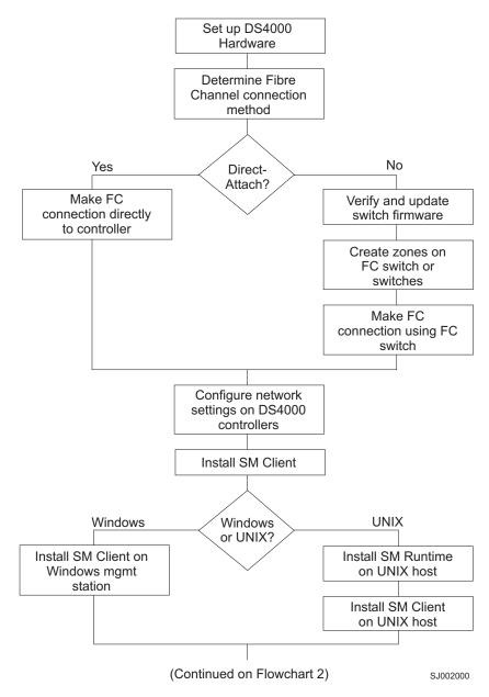
Figure 5. Installation process (part 1)
