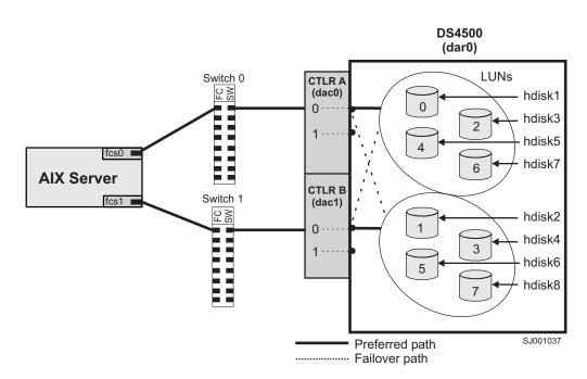
Figure 8. DS4000/AIX system configuration
