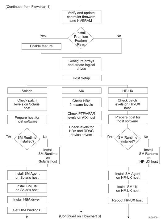
Figure 6. Installation process (part 2)
