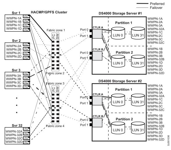
Figure 20. HACMP/GPFS cluster configuration with two DS4000 storage subsystems — two partitions per DS4000
