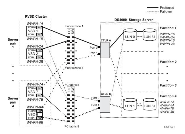
Figure 15 shows a cluster configuration that contains a single DS4000 storage subsystem, with one to four partitions.
