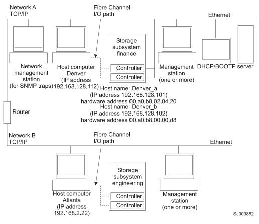
Figure 4. Sample network using both out-of-band and in-band managed storage subsystems
