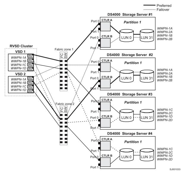
Figure 17. Cluster configuration with four DS4000 storage subsystems — one partition per DS4000
