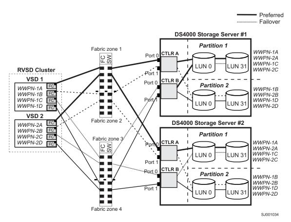
Figure 18. RVSD cluster configuration with two DS4000 storage subsystems — two partitions per DS4000
