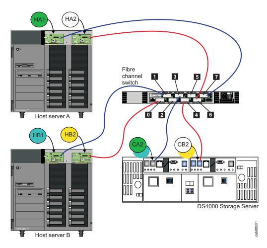
Figure 21. Fibre channel fabric switch environment connecting host servers to a DS4000 Storage Server
