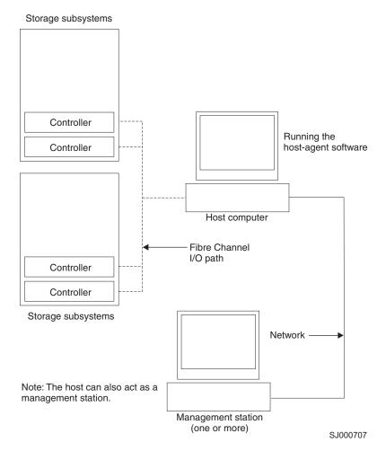
Figure 2. In-band managed storage subsystems
