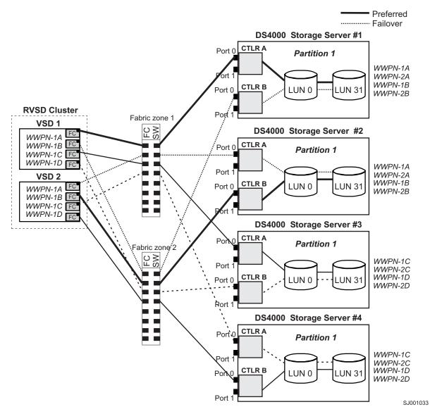
Figure 17. Cluster configuration with four DS4000 storage servers — one partition per DS4000
