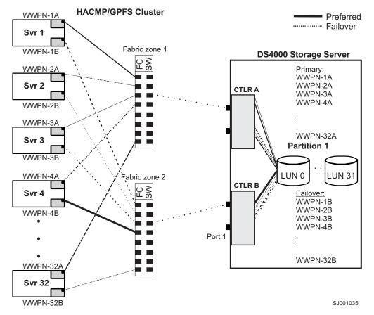
Figure 19. HACMP/GPFS cluster configuration with one DS4000 storage server — one partition
