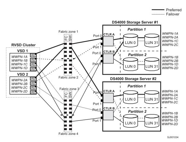
Figure 18. RVSD cluster configuration with two DS4000 storage servers - two partitions per DS4000
