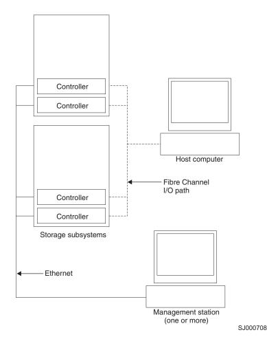
Figure 3. Out-of-band managed storage subsystems
