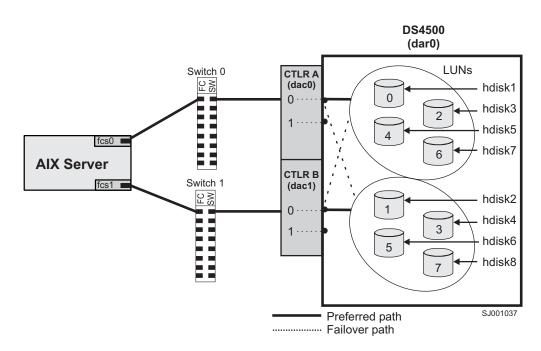
Figure 8. DS4000/AIX system configuration
