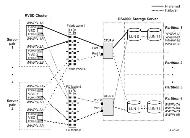
Figure 15. Cluster configuration with single DS4000 storage server — one to four partitions
