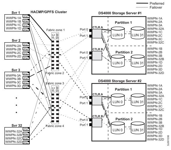
Figure 20. HACMP/GPFS cluster configuration with two DS4000 storage servers — two partitions per DS4000
