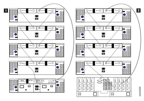
Figure 13. Unacceptable cable loop scheme for connecting DS4000 storage devices
