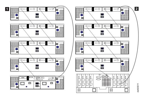
Figure 10. Possible (but not recommended) alternate cable loop scheme for when connecting DS4000 storage devices
