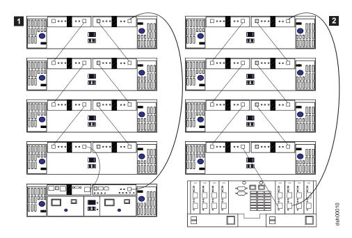
Figure 11. Possible (but not recommended) alternate cable loop scheme for connecting DS4000 storage devices
