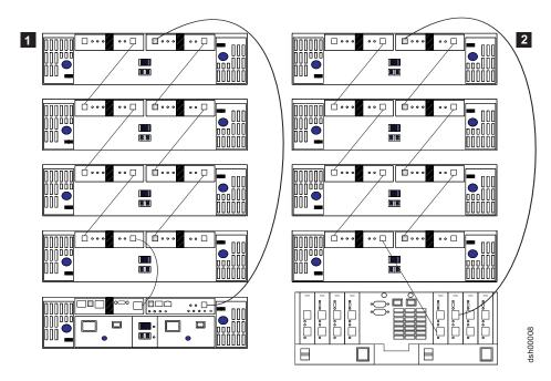
Figure 9. Recommended cable loop scheme for connecting DS4000 storage devices
