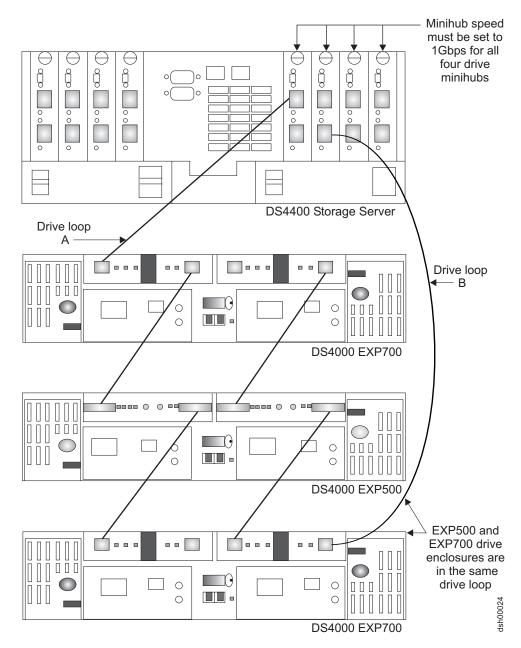
Figure 2. DS4000 EXP500 and EXP700 cabling in a mixed configuration
