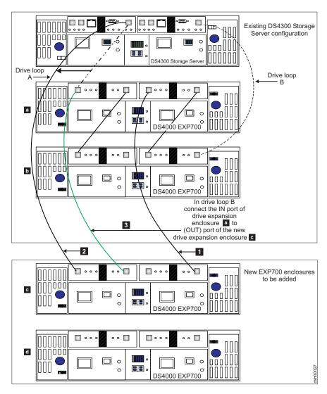
Figure 27. Cabling a single drive enclosure to the beginning of a functioning drive loop (step 3 of 3)
