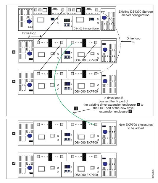
Figure 25. Cabling a single drive enclosure to the beginning of a functioning drive loop (step 1 of 3)
