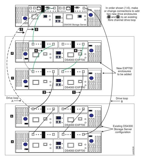
Figure 30. Recommended connection: Planned cabling of additional drive enclosures to the beginning of a functioning drive loop
