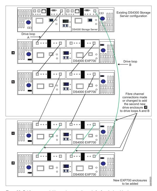
Figure 28. Cabling a second drive enclosure to the end of a functioning drive loop
