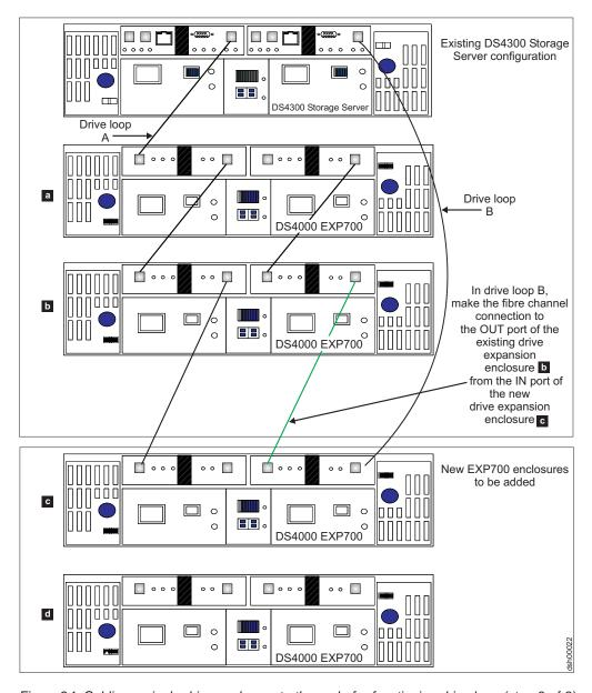
Figure 24. Cabling a single drive enclosure to the end of a functioning drive loop (step 3 of 3)
