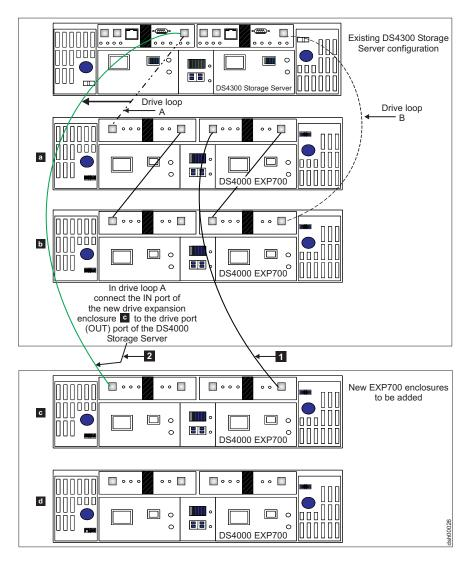
Figure 26. Cabling a single drive enclosure to the beginning of a functioning drive loop (step 2 of 3)
