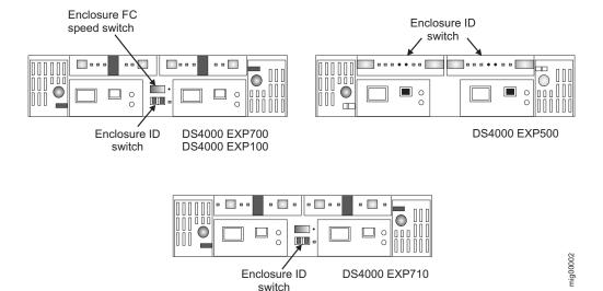
Figure 21. EXP100, EXP500, EXP700, and EXP710 enclosure ID and speed switches
