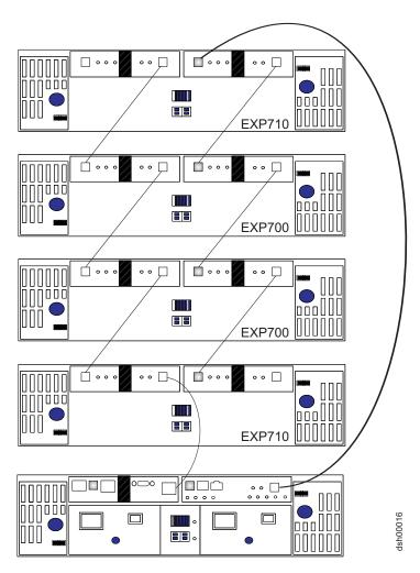
Figure 6. Unacceptable intermixed EXP700 (or EXP100) and EXP710 loop configuration (1 of 2)
