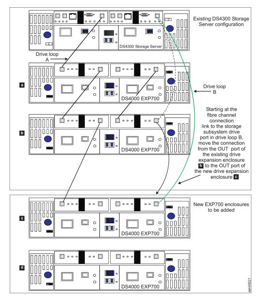
Figure 32. Cabling a single drive enclosure to the end of a functioning drive loop (step 2 of 3)
