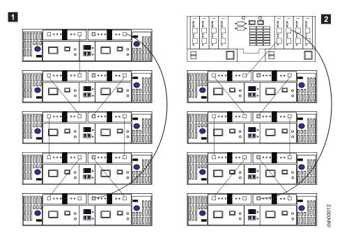
Figure 12. Unacceptable cable loop scheme for connecting DS4000 storage devices
