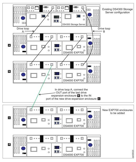
Figure 31. Cabling a single drive enclosure to the end of a functioning drive loop (step 1 of 3)
