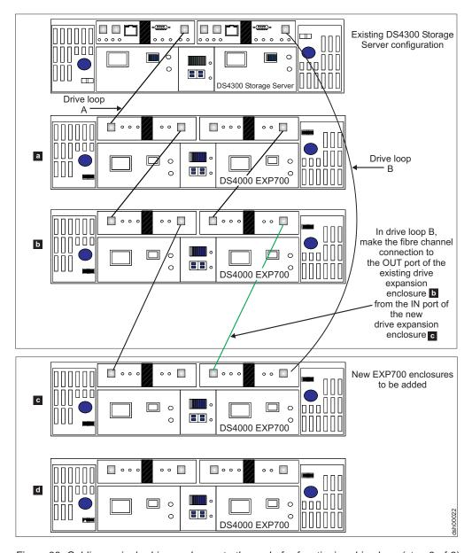
Figure 33. Cabling a single drive enclosure to the end of a functioning drive loop (step 3 of 3)
