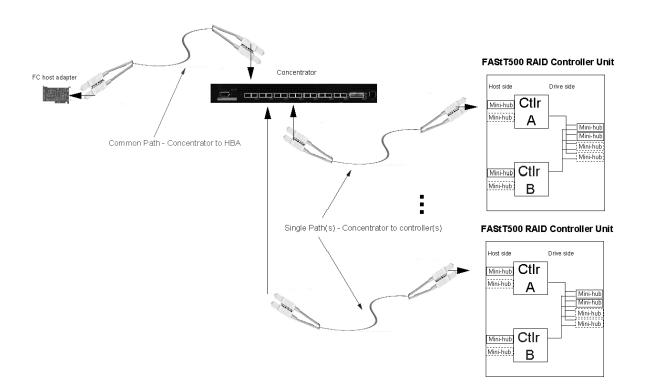
Figure 4. Common path configuration
