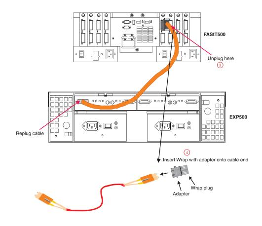
Figure 47. Insert wrap plug with adapter on cable end
