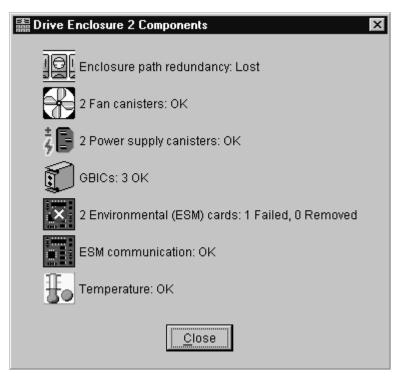
Figure 34. Drive enclosure components - ESM failure
