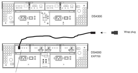
Record status of bypass light after wrap plug is inserted.
