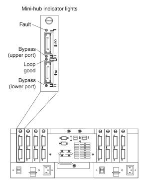
Figure 38. FAStT500 RAID controller mini-hub indicator lights
