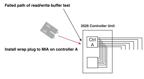
Figure 59. Install wrap plug to MIA
