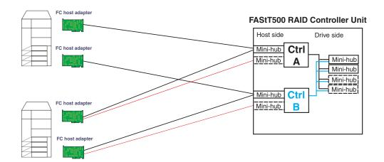
Figure 10. Type 2 configuration - Without hubs
