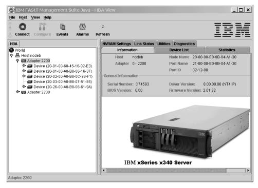
Figure 21. FAStT MSJ window - One 2200 host adapter
