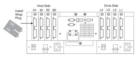
Figure 18. Install wrap plug to GBIC or SFP in mini-hub on controller A
