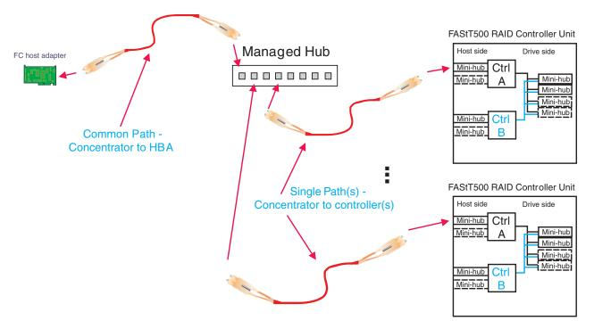
Figure 11. Type 2 configuration with multiple controller units
