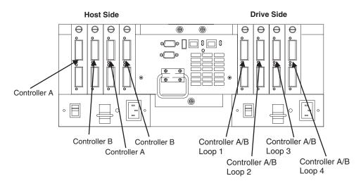
Figure 27. FAStT500 controller connection locations
