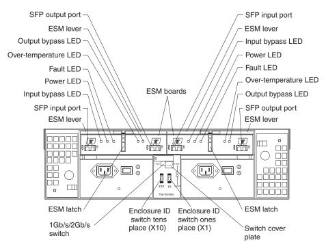
Figure 44. DS4000 EXP700, DS4000 EXP710, and DS4000 EXP100 ESMs and user controls
