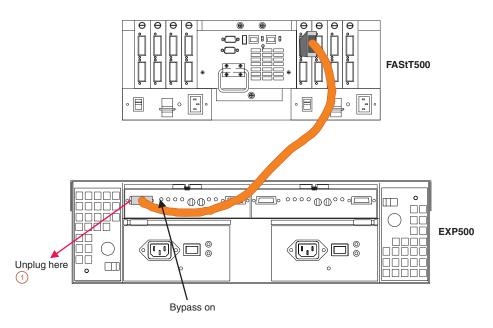
Figure 45. Disconnect cable from loop element
