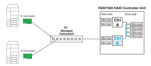
Figure 13. All I/O flowing through controller A
