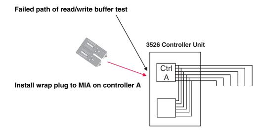
Figure 17. Install wrap plug to MIA on controller A
