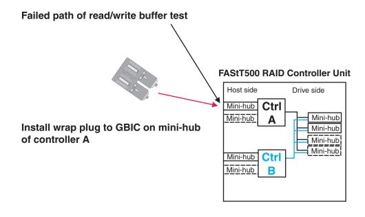
Figure 58. Install wrap plug to GBIC
