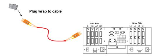
Figure 19. Install wrap plug
