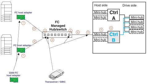
Figure 14. Path elements loop
