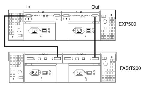
Figure 29. EXP500 and FAStT200 configuration
