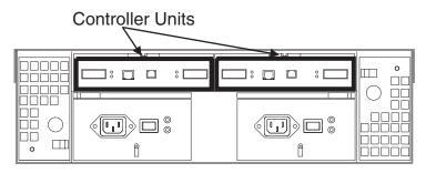
Figure 28. FAStT200 fibre channel controller unit locations
