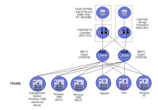
Figure 64. Heterogeneous configuration
