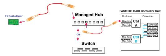
Figure 55. Typical connection path
