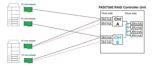
Figure 9. Type 2 configuration - With hubs
