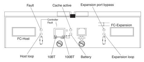
Figure 37. FAStT200 controller indicator lights
