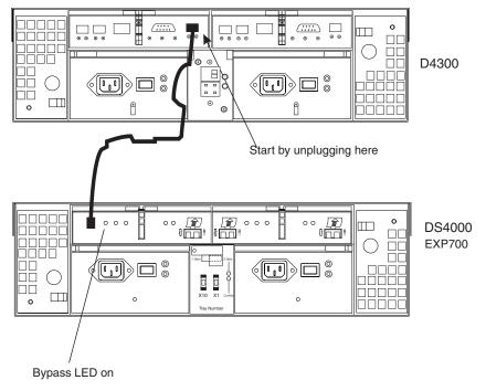
Figure 49. Copper cable and bypass light
