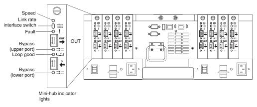
Figure 39. Type 1742 DS4400 Storage Server mini-hub indicator lights
