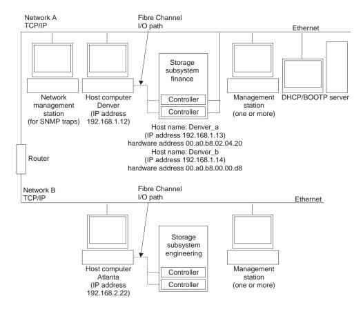
Figure 5. Sample network using direct and host-agent managed storage subsystems
