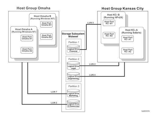
Figure 12. Storage partitioning example
