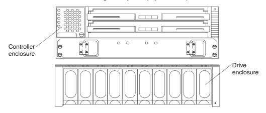
Figure 2. Storage subsystem physical components
