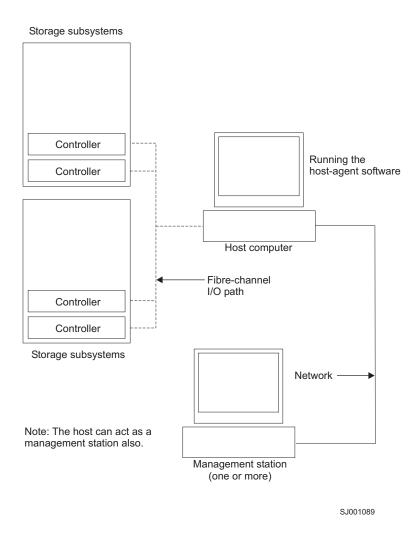
Figure 4. Host-agent (in-band) managed storage subsystems
