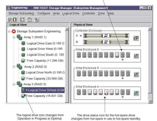
Figure 24. Recovery Guru window showing Optimal status
