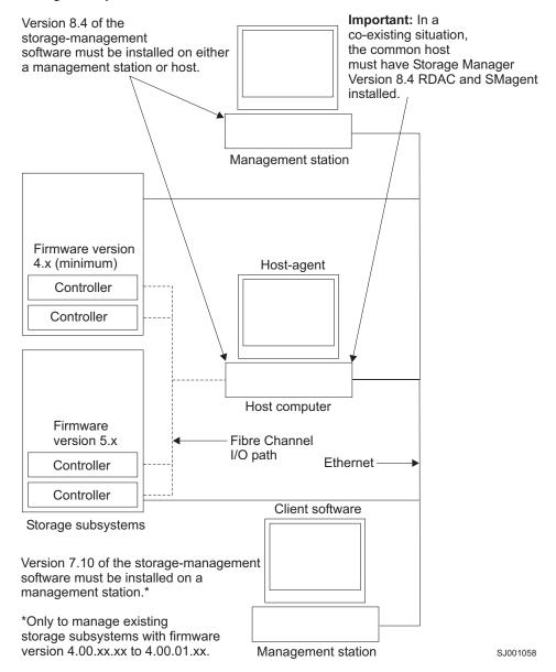
Figure 6. Sample coexisting storage subsystems
