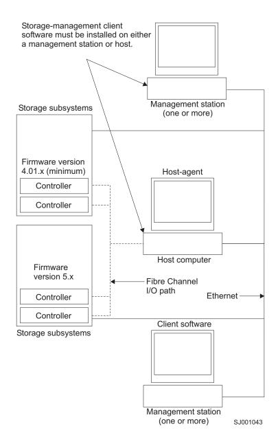
Figure 6. Coexisting storage subsystems
