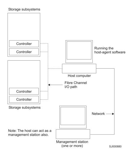
Figure 2. Host-agent (in-band) managed storage subsystems
