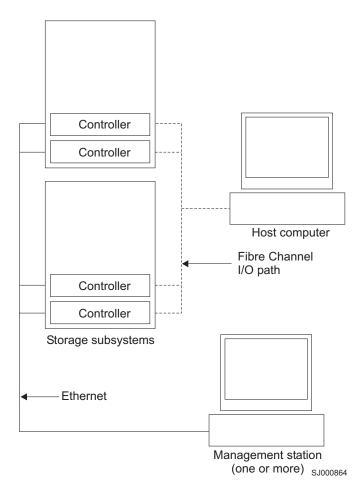
Figure 2. Direct (out-of-band) managed storage subsystems
