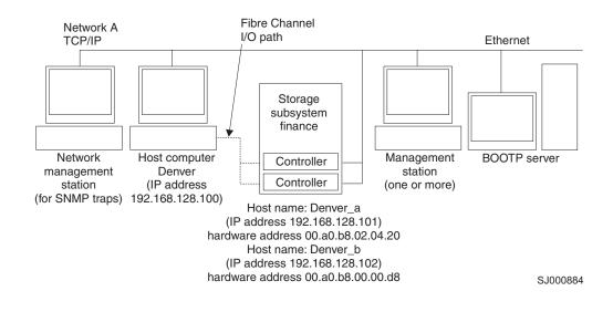
Figure 5. Sample network using direct-managed storage subsystems
