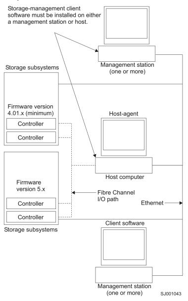
Figure 4. Coexisting storage subsystems
