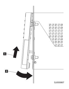
Figure 8. Replacing the controller-unit bezel (machine types 3552 and 1742)
