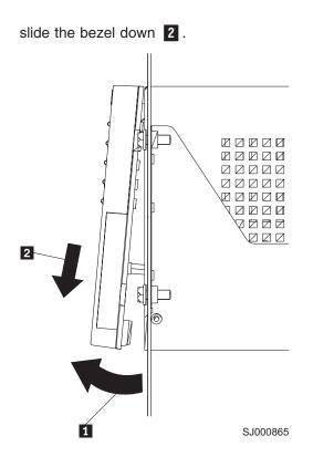
Figure 7. Removing the controller-unit bezel (machine types 3552 and 1742)
