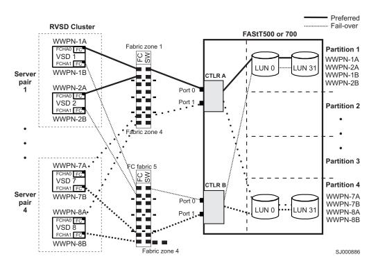
Figure 14. RVSD cluster configuration example with a single FAStT500 or FAStT700, shown with two partitions (four maximum) per FAStT
