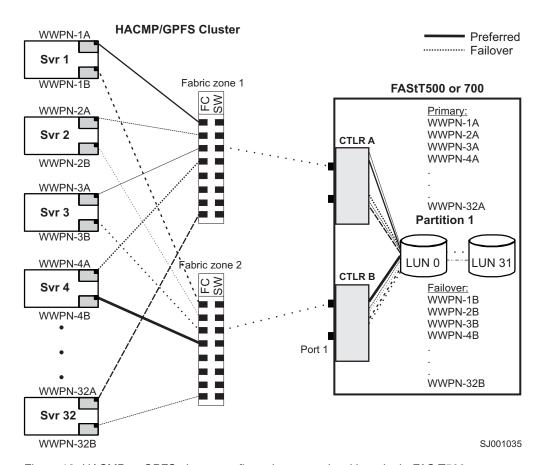
Figure 18. HACMP or GPFS cluster configuration example with a single FAStT500 or FAStT700, shown with one partition per FAStT
