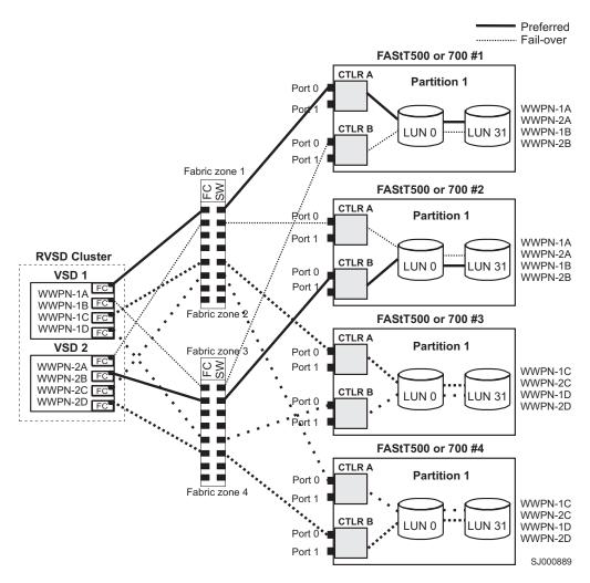
Figure 17. Typical RVSD cluster configuration example with multiple FAStT500 or FAStT700, shown with one partition per FAStT
