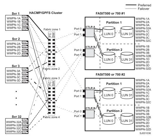
Figure 19. HACMP or GPFS cluster configuration example with multiple FAStT500 or FAStT700, shown with two partitions per FAStT
