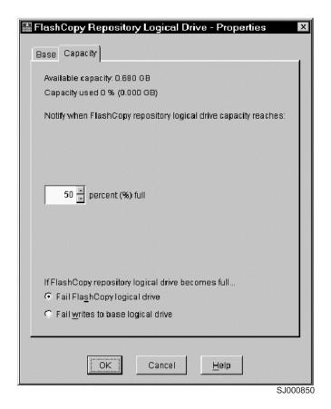
Figure 45. Repository drive warning threshold
