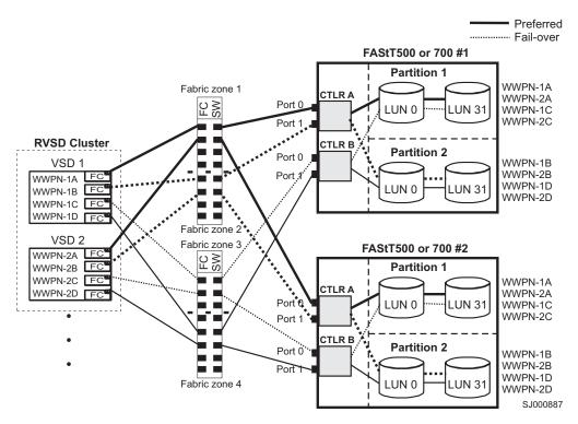
Figure 15. RVSD cluster configuration example with multiple FAStT500 or FAStT700, shown with two partitions per FAStT
