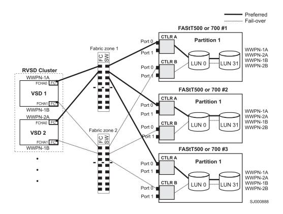
Figure 16. RVSD cluster configuration example with multiple FAStT500 or FAStT700, shown with one partition per FAStT
