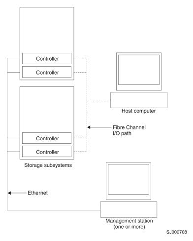
Figure 3. Direct (out-of-band) managed storage subsystems
