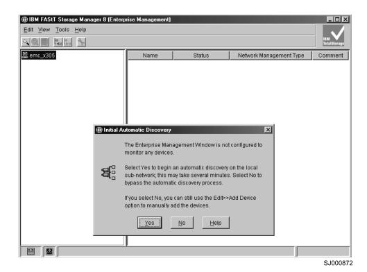
Figure 18. Confirm Initial Automatic Discovery window
