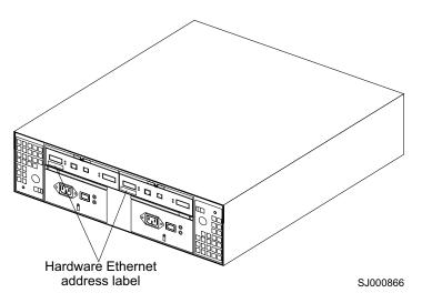
Figure 8. Locating the Ethernet MAC address for machine type 3542 and 1722
