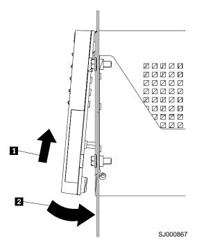
Figure 10. Replacing the controller-unit bezel (machine types 3552 and 1742)
