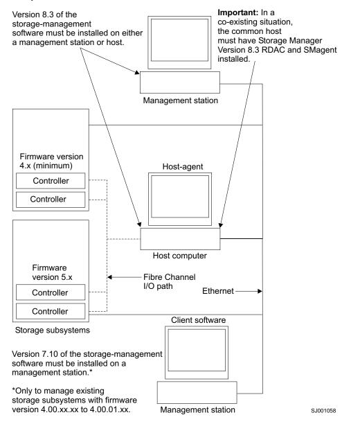
Figure 7. Sample coexistent installation
