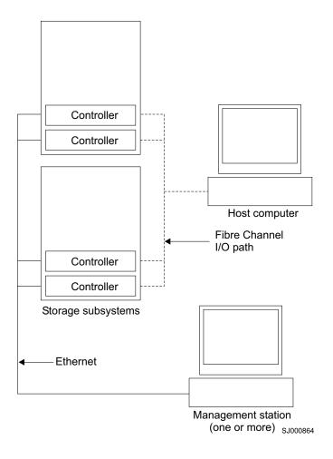
Figure 3. Direct-management (out-of-band) storage subsystems
