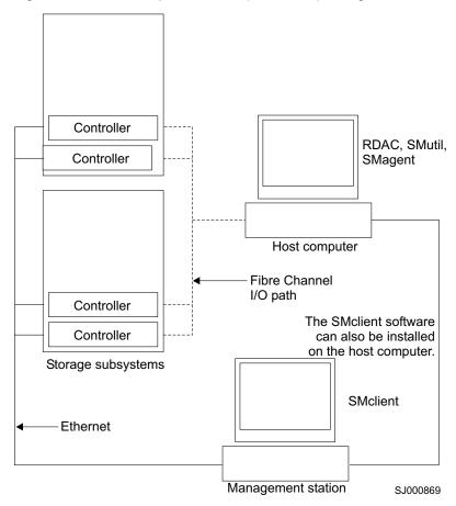
Figure 5. Sample standard (noncluster) configuration
