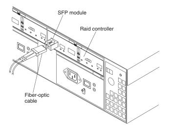
Figure 68. Location of SFPs and fiber-optic cables
