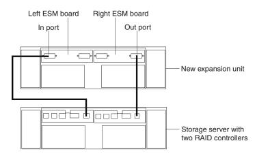
Figure 41. Adding an expansion unit
