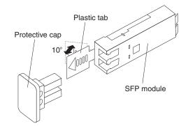
Figure 50. Unlocking the SFP module latch - plastic variety
