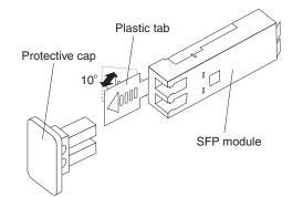
Figure 69. Unlocking the SFP module latch - plastic variety
