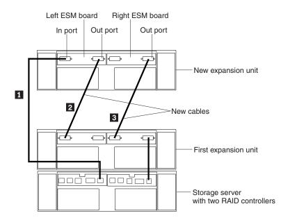
Figure 42. Adding a second expansion unit
