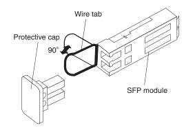
Figure 33. Unlocking the SFP module latch - wire variety
