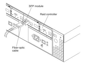
Figure 35. Connecting cables to the installed SFP
