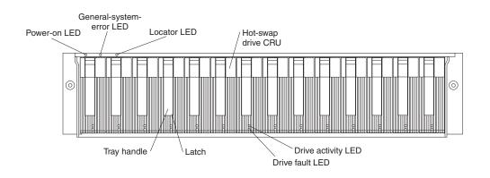
Figure 2. Front controls and components
