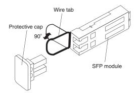
Figure 70. Unlocking the SFP module latch - wire variety
