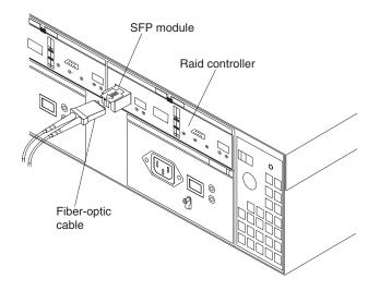
Figure 54. Location of SFPs and fiber-optic cables
