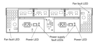
Figure 45. Fan and power supply LEDs
