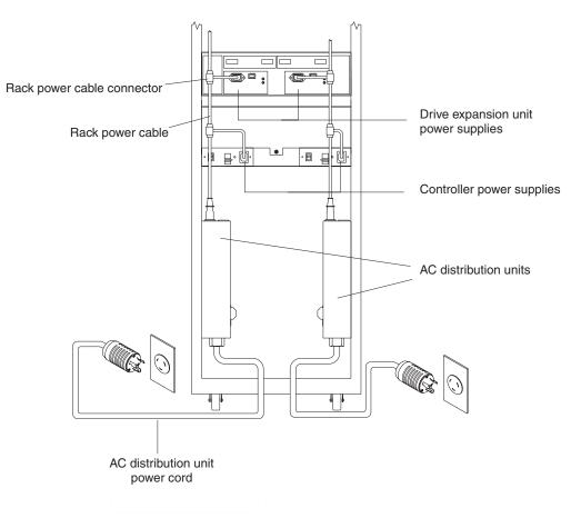
Figure 40. Redundant ac power connections to controllers and drive expansion units
