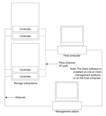
Figure 20. Direct-managed storage subsystems
