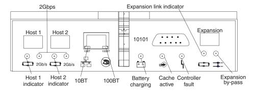
Figure 44. RAID controller LEDs
