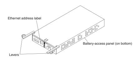
Figure 48. RAID controller levers and labels
