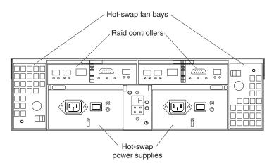
Figure 3. Back view of FAStT600 storage server (Model 60U/60X)
