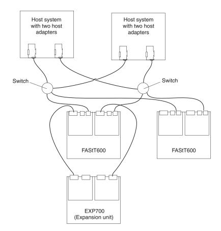
Figure 23. Example of a dual-SAN fabric zone configuration (Model 60U/60X)
