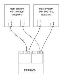
Figure 21. Redundant host and drive Fibre Channel loop configurations (Model 60U/60X)
