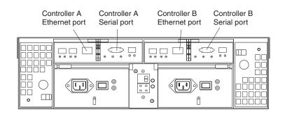
Figure 38. Ethernet and serial port locations
