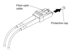
Figure 34. Removing caps from fiber-optic cables
