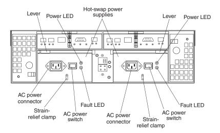
Figure 63. Power supply controls
