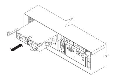
Figure 52. Pull-rings for removing a controller
