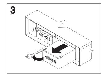
Figure 12. Power supply removal
