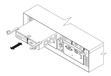
Figure 71. Pull-rings for removing a controller
