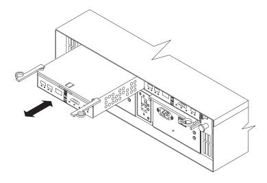
Figure 57. Pull-rings for removing a controller
