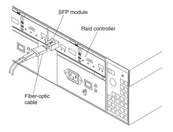
Figure 49. Location of SFPs and fiber-optic cables
