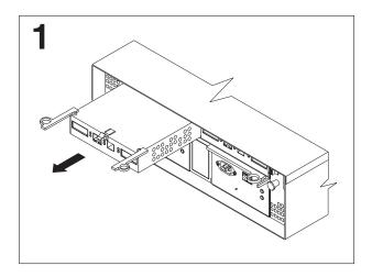
Figure 10. RAID controller removal
