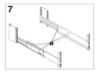
Figure 16. Rail adjustment screws
