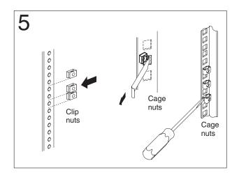
Figure 14. Rack nut installation
