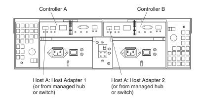
Figure 36. Location of host cables (Model 60U/60X)
