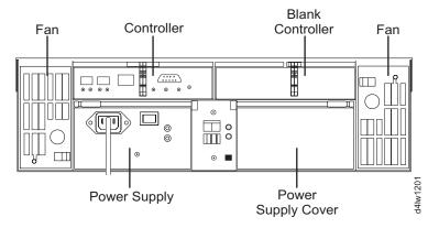
Figure 4. Back view of FAStT600 storage server (Model 6LU/6LX)
