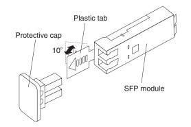
Figure 32. Unlocking the SFP module latch - plastic variety
