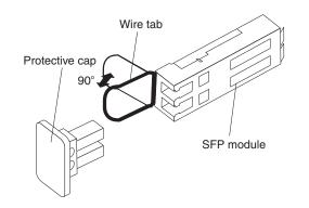
Figure 56. Unlocking the SFP module latch - wire variety
