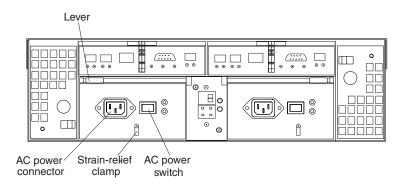
Figure 66. Connecting the power cord to the AC power connector
