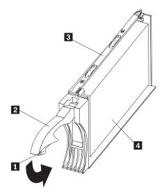
Figure 59. Releasing the drive latch
