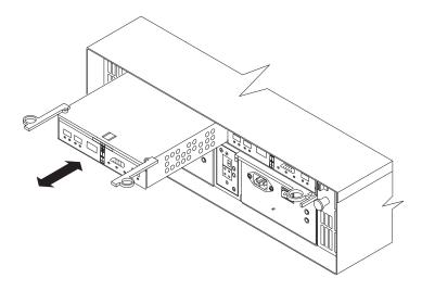
Figure 74. Installing a new RAID controller
