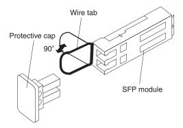
Figure 52. Unlocking the SFP module latch - wire variety
