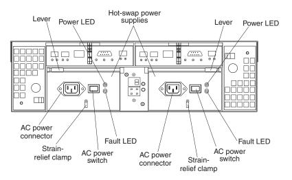
Figure 45. Power supply controls
