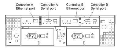
Figure 30. Ethernet and serial port locations
