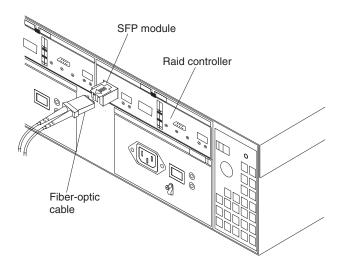
Figure 50. Location of SFPs and fiber-optic cables
