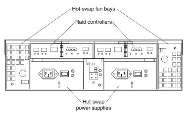
Figure 3. Back view of FAStT600 storage server
