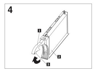
Figure 11. Hard disk drive removal
