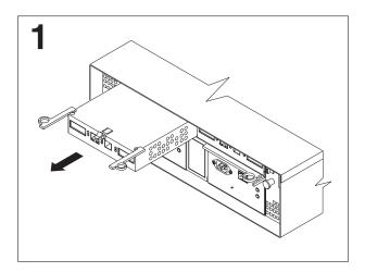
Figure 8. RAID controller removal
