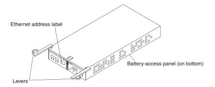
Figure 49. RAID controller levers and labels
