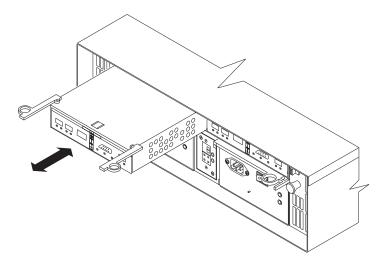
Figure 53. Pull-rings for removing a controller
