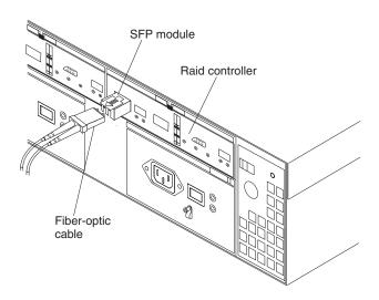
Figure 28. Connecting cables to the installed SFP
