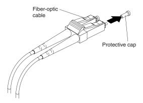
Figure 27. Removing caps from fiber-optic cables
