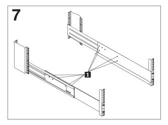
Figure 14. Rail adjustment screws
