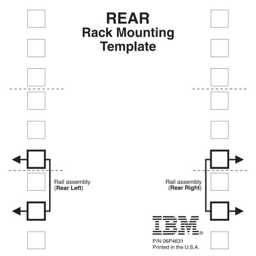
Figure 7. Rear rack mounting template
