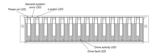
Figure 35. Storage server LEDs (front)
