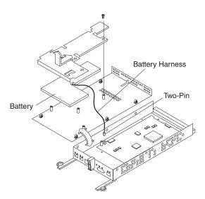
Figure 55. Removing the controller battery
