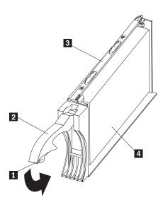
Figure 41. Releasing the drive latch
