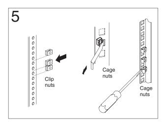
Figure 12. Rack nut installation
