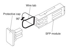
Figure 26. Unlocking the SFP module latch - wire variety
