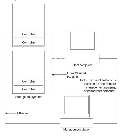
Figure 18. Direct-managed storage subsystems
