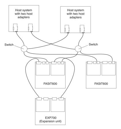
Figure 21. Example of a dual SAN fabric zone configuration
