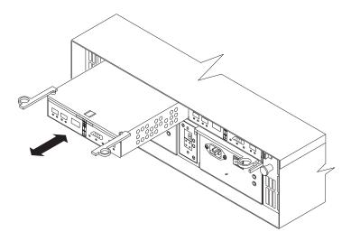
Figure 56. Installing a new RAID controller
