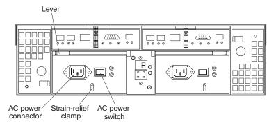
Figure 46. Lever for power supply removal
