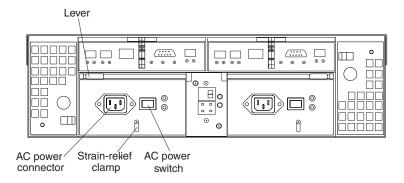
Figure 48. Connecting the power cord to the AC power connector
