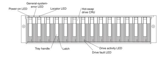
Figure 2. Front controls and components
