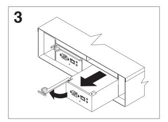
Figure 10. Power supply removal
