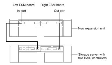
Figure 33. Adding an expansion unit
