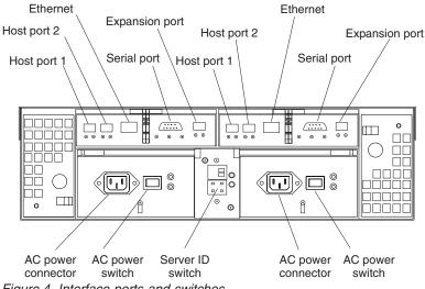
Figure 4. Interface ports and switches
