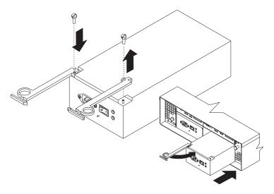
Figure 47. Installing a hot-swap power supply
