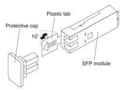
Figure 51. Unlocking the SFP module latch - plastic variety
