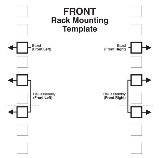
Figure 6. Front rack mounting template
