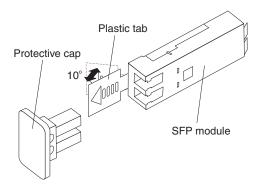
Figure 25. Unlocking the SFP module latch - plastic variety
