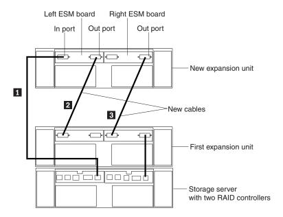
Figure 34. Adding a second expansion unit
