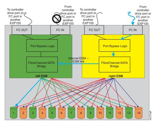
Figure 46. The right ESM and controller firmware recover from a loss of connectivity to the input port of the left ESM
