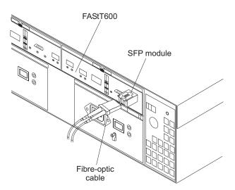
Figure 32. Connecting cables to the installed SFP
