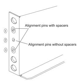
Figure 11. Alignment pins with and without spacers
