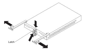
Figure 42. Removing the failed ESM
