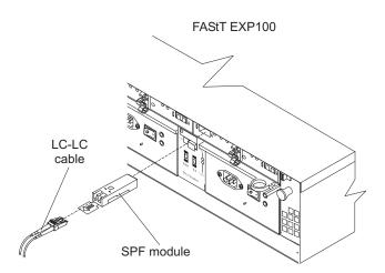
Figure 35. Installing an SFP module and connecting an LC-LC cable to the FAStT EXP100
