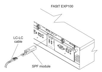
Figure 33. Installing an SFP module and connecting an LC-LC cable to the FAStT EXP100
