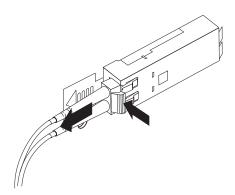
Figure 31. Removing the LC-LC fibre-channel cable
