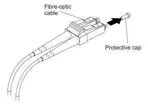
Figure 28. Removing fiber-optic cable protective caps
