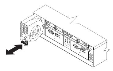
Figure 43. Replacing a hot-swap cooling fan
