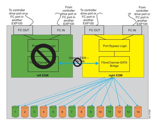
Figure 47. Right ESM reroutes I/Os along dashed alternate paths
