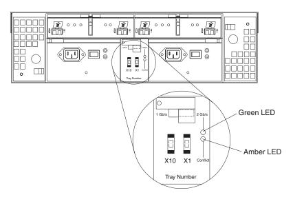
Figure 21. Enclosure ID switches
