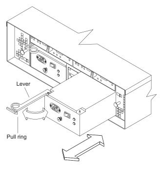
Figure 19. Replacing a power supply
