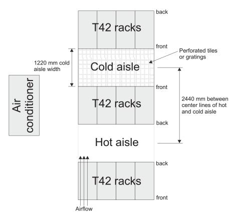
Figure 8. Example of cold aisle/hot aisle rack configuration
