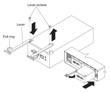
Figure 40. Moving the power supply lever and replacing the failed hot-swap power supply
