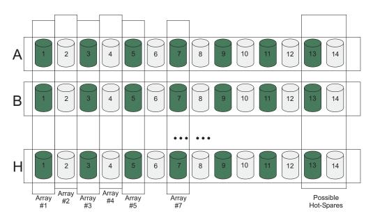
Figure 48. Orthogonally striped RAID arrays - Option 1
