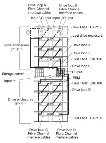
Figure 37. Cabling the FAStT EXP100 to two redundant loops
