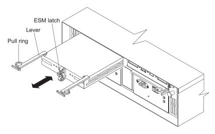
Figure 18. Replacing an ESM
