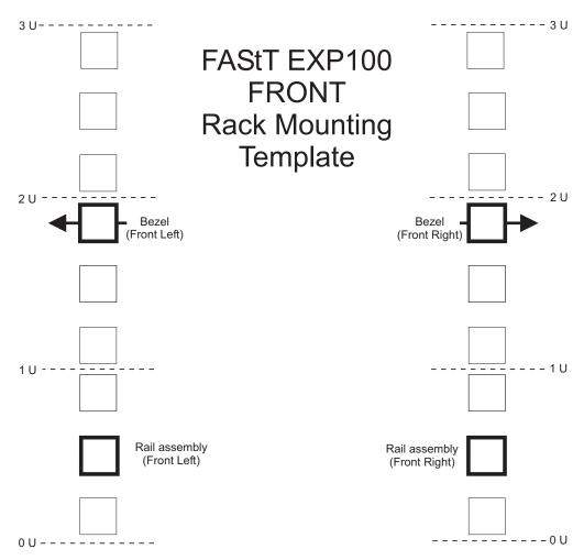
Figure 50. Front rack mounting template
