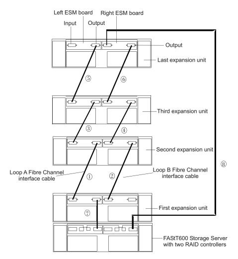
Figure 36. FAStT EXP100 redundant loop configuration
