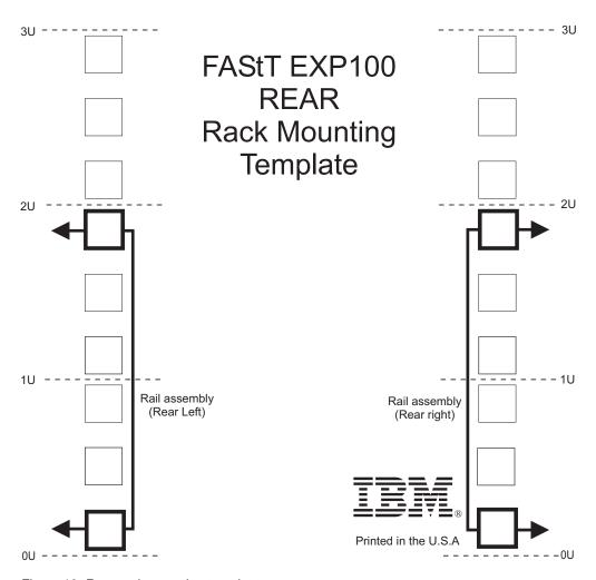
Figure 10. Rear rack mounting template
