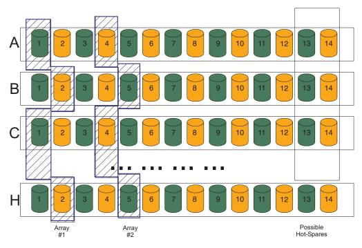
Figure 49. Orthogonally striped RAID arrays - Option 2
