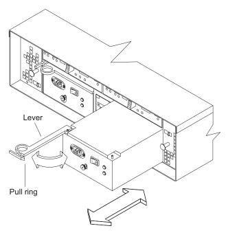
Figure 14. Removing a power supply
