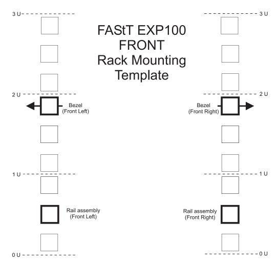
Figure 9. Front rack mounting template
