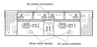
Figure 41. Connecting the power supply
