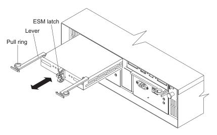
Figure 13. Removing an ESM
