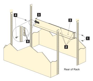
Figure 12. Installing the support rails
