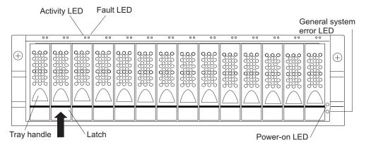
Figure 38. Hot-swap hard disk drive LEDs
