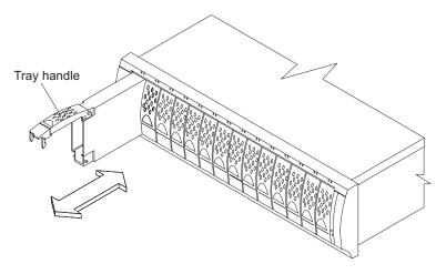
Figure 16. Removing a drive CRU
