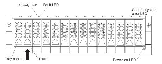
Figure 4. Front controls and indicators
