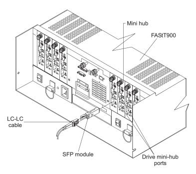
Figure 34. Installing an SFP module and LC-LC cable in a FAStT900
