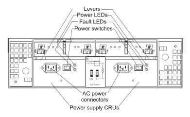
Figure 5. Power supply controls, indicators, and connectors
