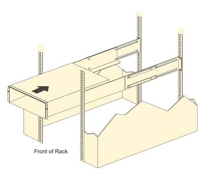
Figure 17. Installing the FAStT EXP100
