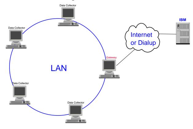
Electronic Service Agent is installed on every system you want monitored. Each system being monitored is designated as a Data Collector, and one system within your network is designated as a Gateway, which is also considered a managed system. The Data Collector gathers information about your system and forwards it to the Gateway. The Gateway machine formats all the information and sends the collected data to IBM, either by dial-up or via the Internet.
